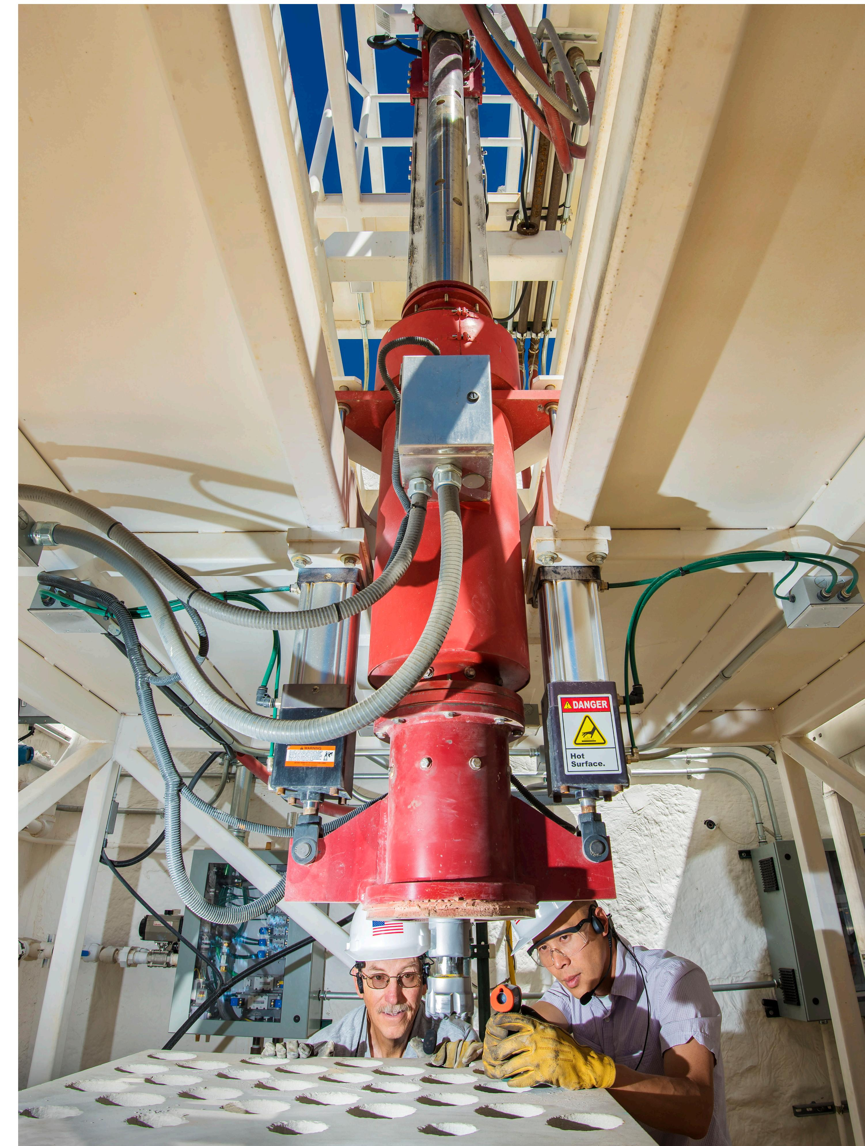
The down-the-hole hammer used in high-temperature environments can help increase the drilling rates and the rate of penetration to maybe five to 10 times that of conventional drilling operations.
