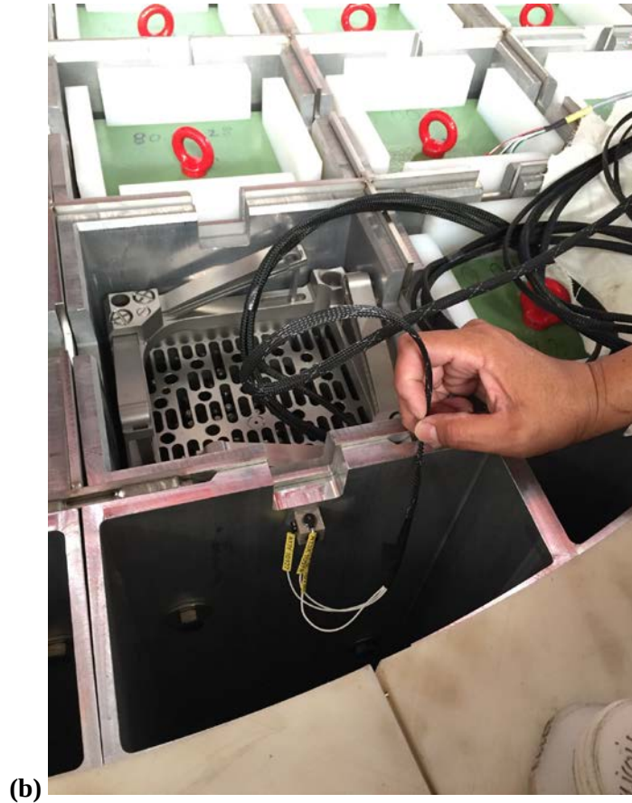
Figure 3-24. Triaxial accelerometer on basket wall adjacent to instrumented surrogate fuel assembly.
