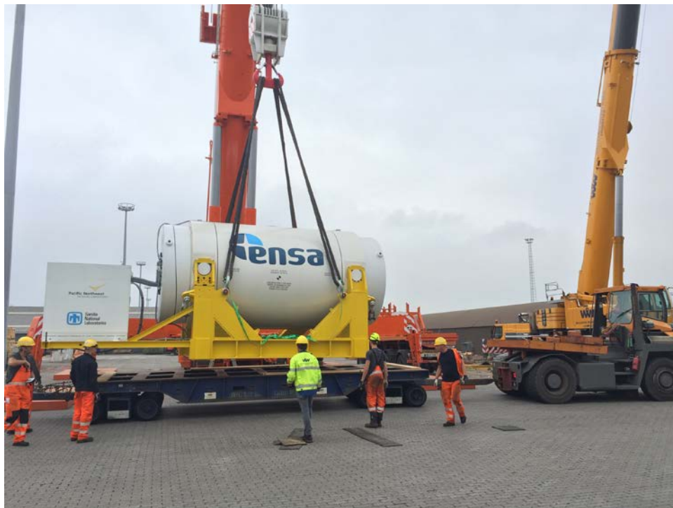
Figure 4-31. Cask system being placed onto Samson at Port of Zeebrugge for transport to Port of Baltimore.
