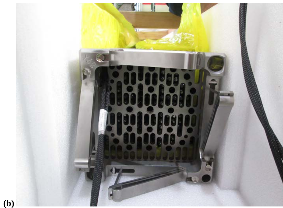
Figure 3-19. The biaxial accelerometer mounted inside the top nozzle of the Korean assembly (a) and the cable leads from the biaxial accelerometer (b).
