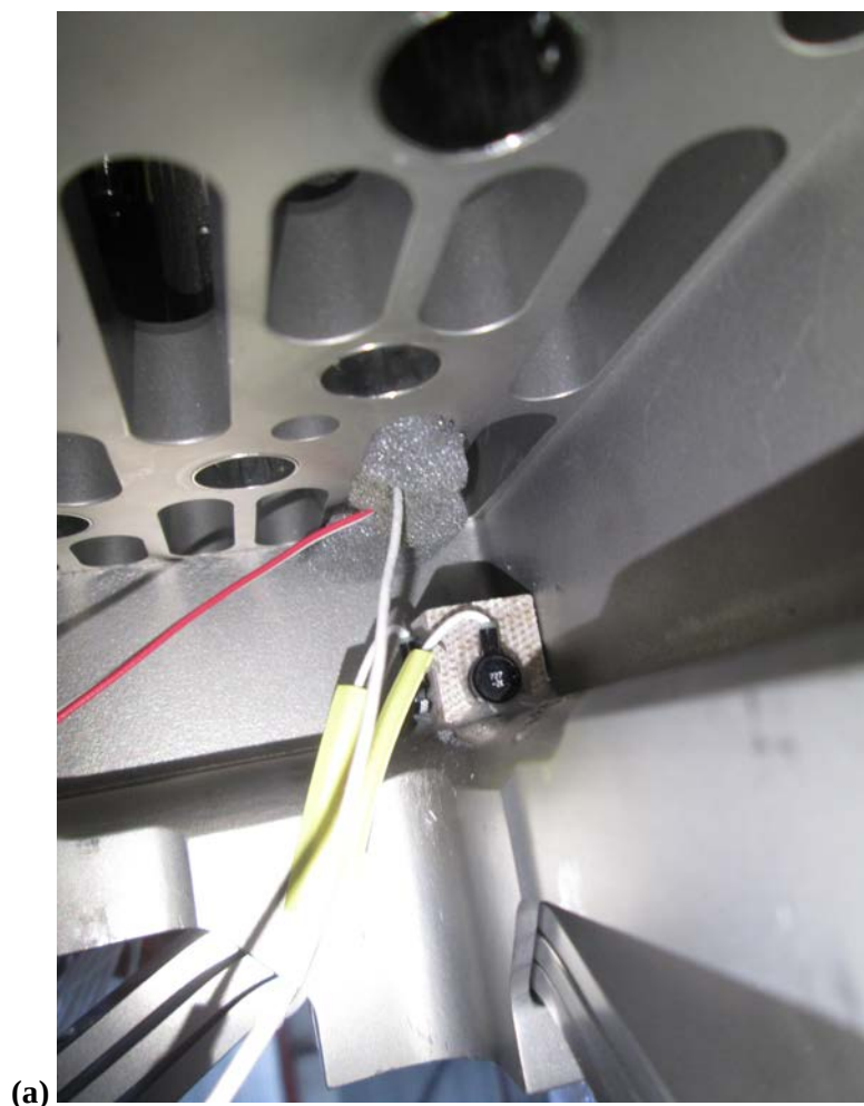
Figure 3-18. The biaxial accelerometer mounted on the top nozzle of the Korean assembly.
