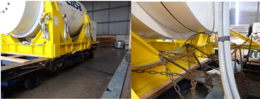
Typical lashing between cradle and SAMSON
