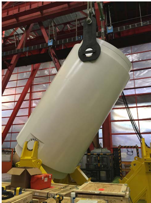
Figure 3-38. Cask being rotated to horizontal position on cradle.
