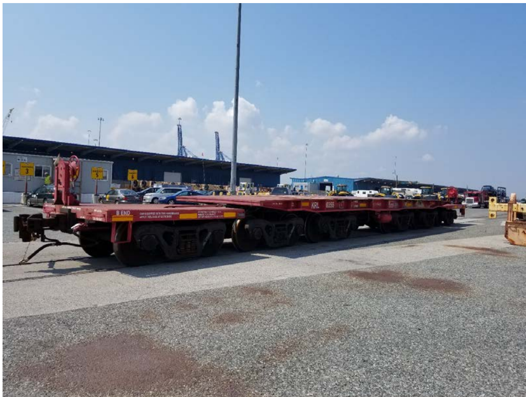
Figure 4-38. Kasgro KRL 370355 flat deck railcar used for the rail tests.
