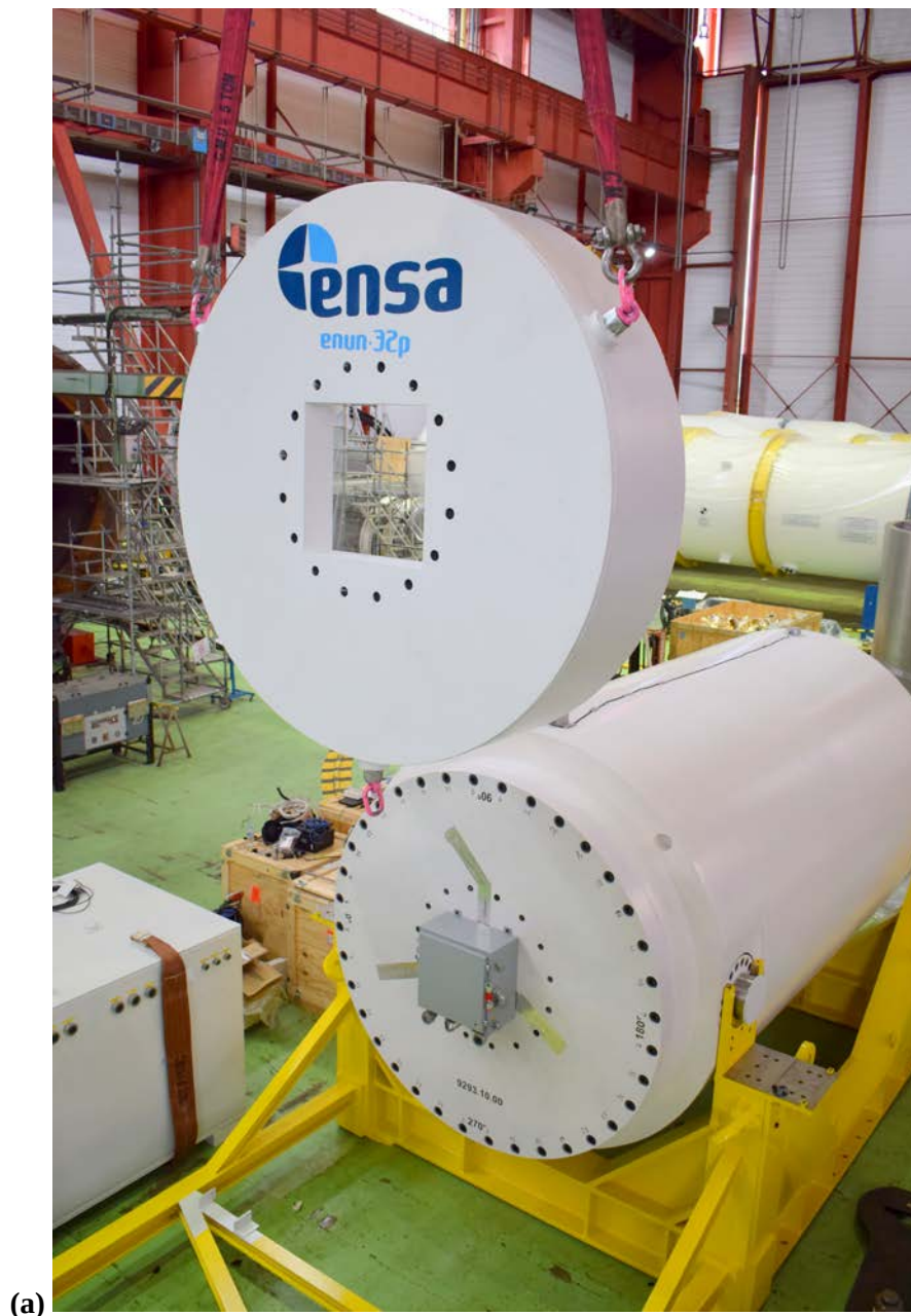
Figure 3-9. Surrogate impact limiter (top) being installed on the test lid (bottom). The gray box is the Junction Box for the instrumentation cables exiting the interior of the cask.
