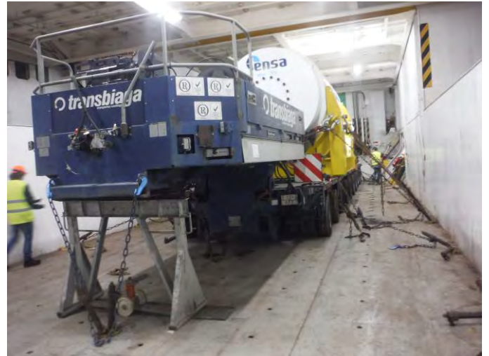
14. General view of lashing in starboard side
