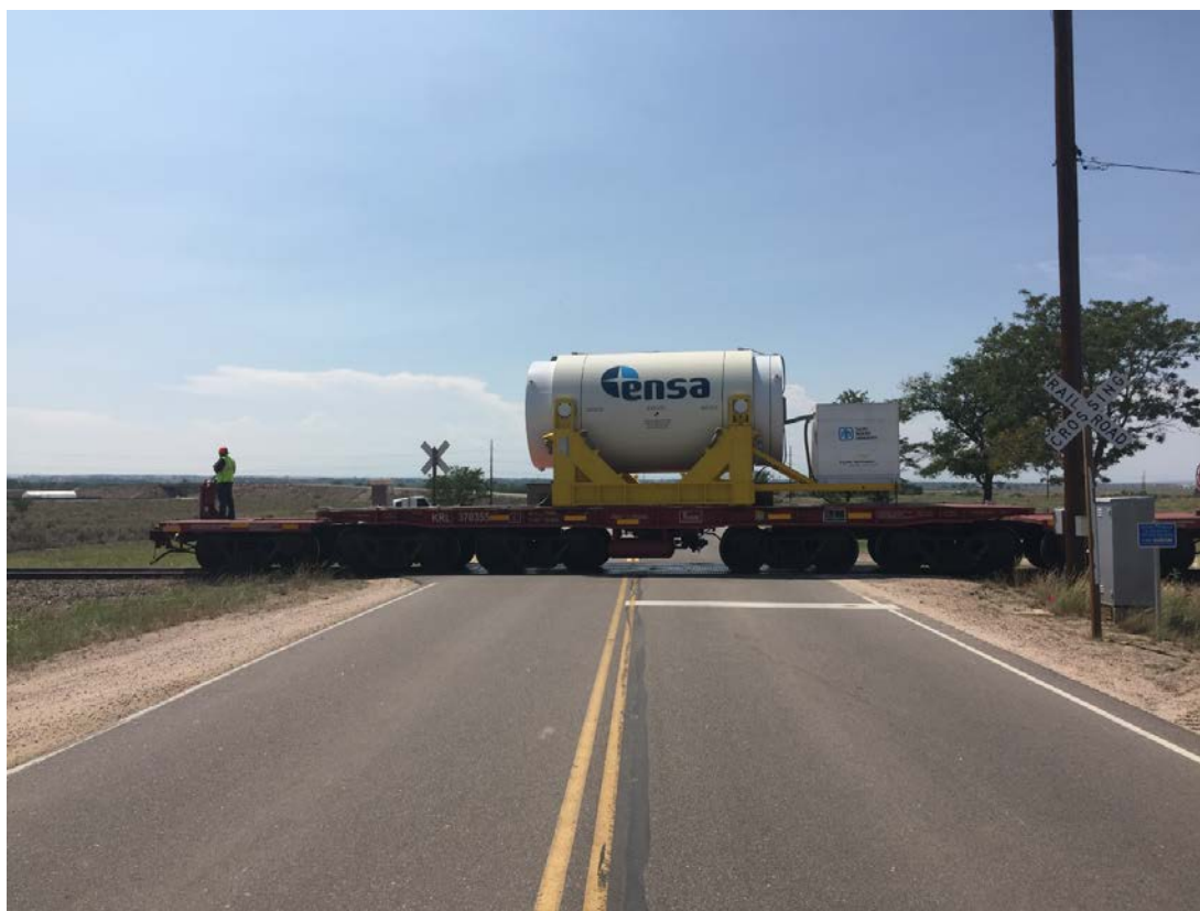
Figure 4-52. Cask being transferred to BNSF rail line from TTCl.
