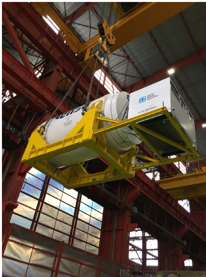
Figure 4-7. Moving cask system to Heavy-Haul Truck Trailer.
