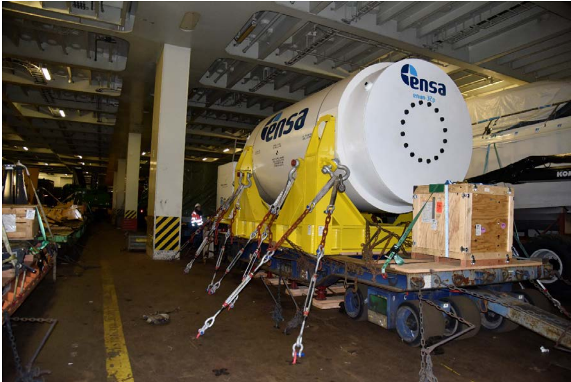
Figure 4-35. Cask lashed to the interior deck of the “Tarago.”
