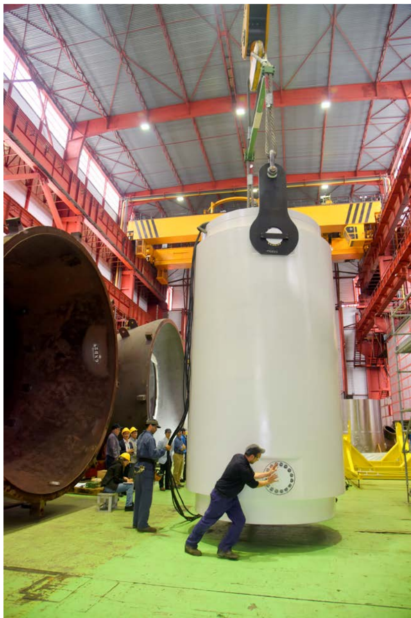
Figure 4-2. Positioning of the cask for Handling Test simulating vertical positioning of cask onto a storage pad.
