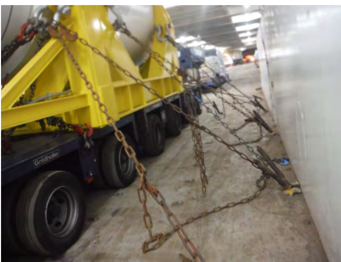
11. Lashing from cradle to deck
