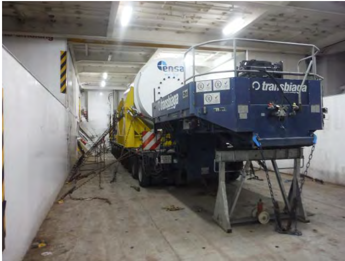
13. General view of lashing in portside
