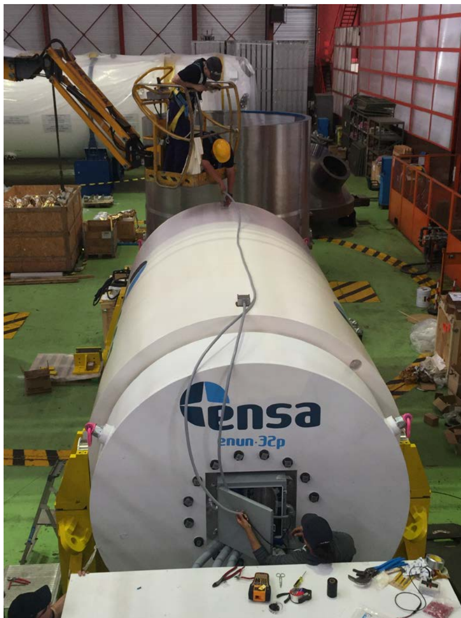
Figure 3-40. ENSA and SNL staff attaching triaxial accelerometers to exterior surface of the cask.
