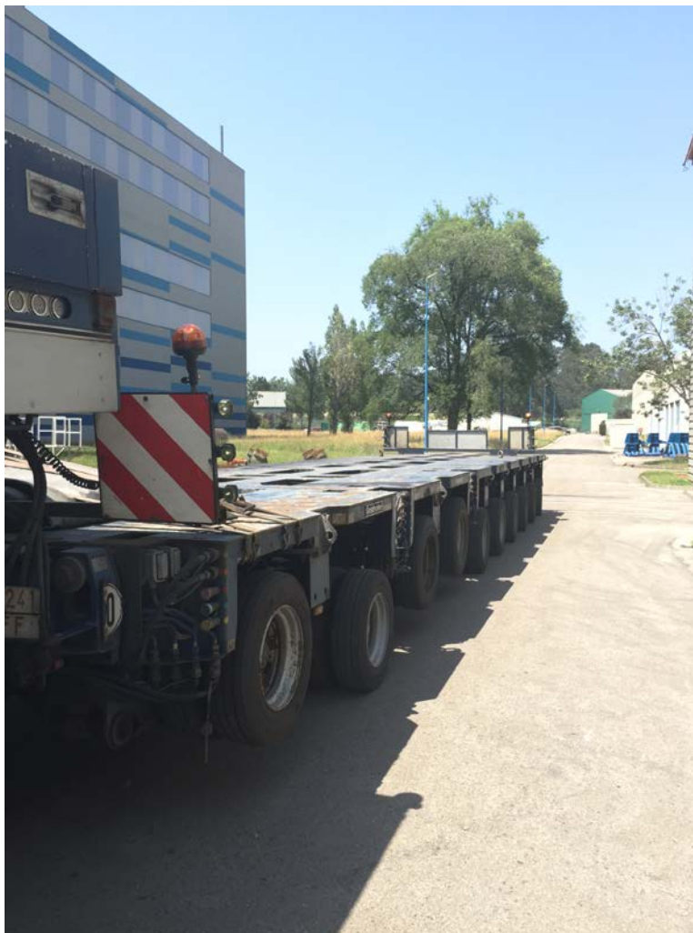
Figure 4-24. 10-axle truck trailer used for Roll-on/Roll-off ship transport from Santander to Zeebrugge.
