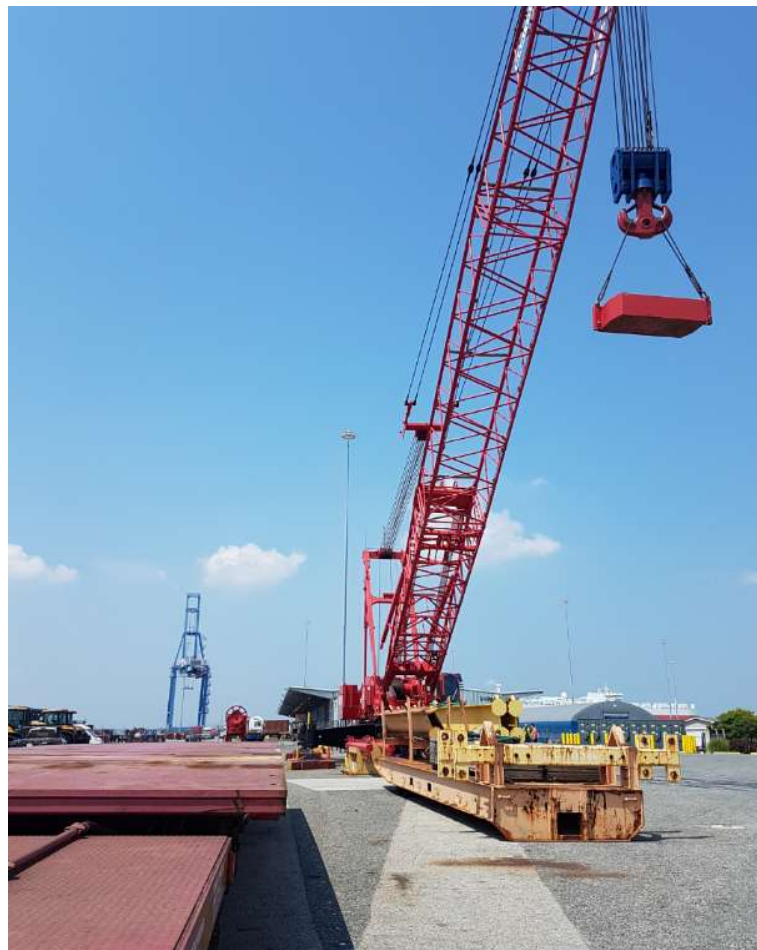
Image 2. Crane of 500Mt capacity.
