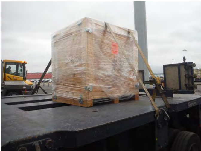
3. Lashing with slings wooden box
