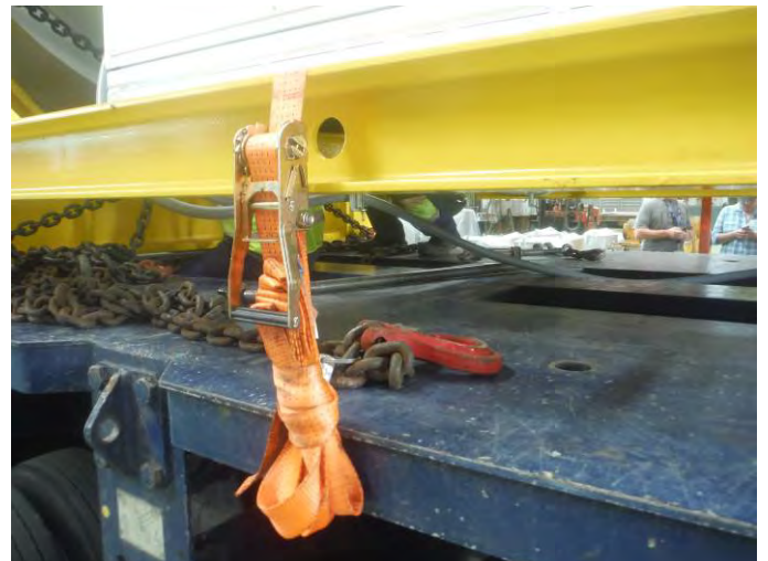
4. Lashing with slings cradle to platform
