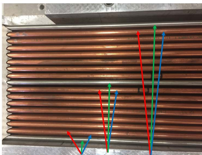
Figure 3-15. The Zircaloy rods (green arrows) were removed from the SNL assembly for reconfiguration for the tests. (The configuration shown in the figure is that for the previous multi-axis shaker tests.) The adjacent copper rods (red arrows) in the top row, and the copper rods in the second row directly below those top-row copper rods, were also removed. The Zircaloy rods were then placed in the second row below the vacant top-row position (blue arrows). The previous positions of the relocated Zircaloy rods were populated with a copper rod. So, the position of the of the Zircaloy rods for the rail-cask tests (blue arrows) was in the second row; there was no rod above the Zircaloy rods.
