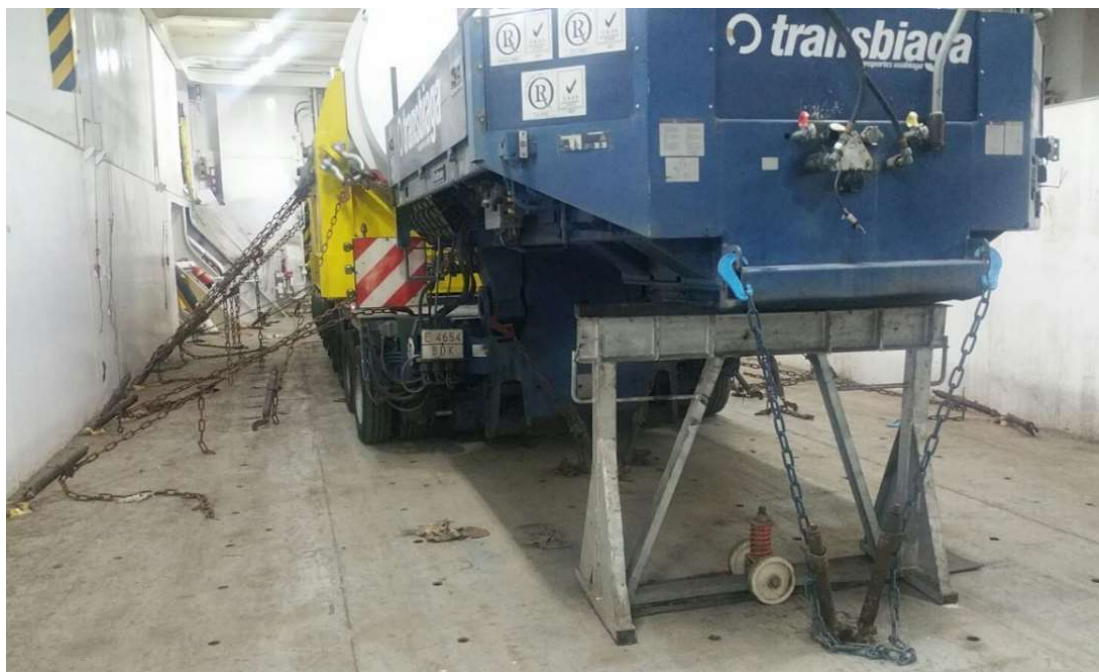
Image 6. Truck platform and cask on board MV Autosky, lashed and secured to vessel deck.
