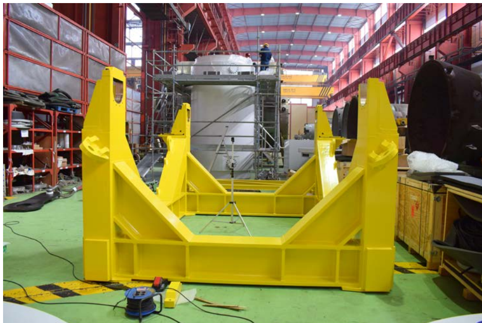
Figure 3-3. ENUN 32P cask basket (a) and its insertion into cask (b).
