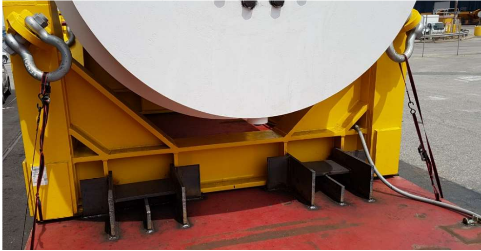
Image 17. 2x stoppers in the back side of CASK.
