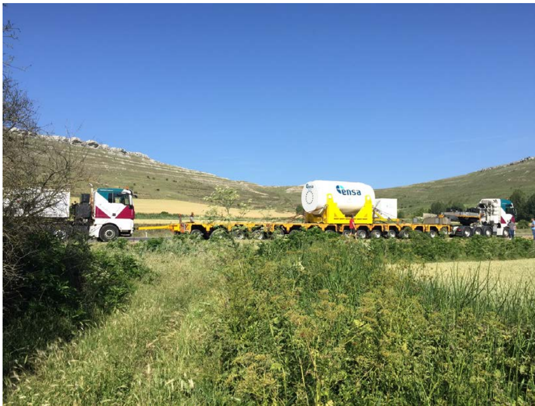
Figure 4-20. Overnight location of cask system near Ubierna. Truck to left in photograph was used to assist in pushing the cask system up hills.
