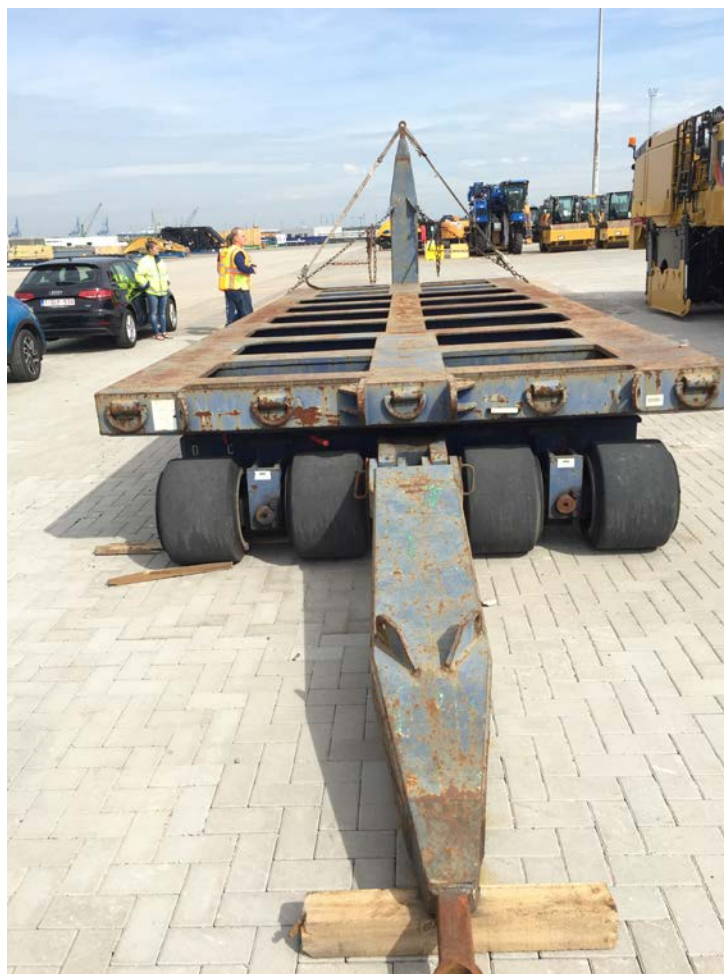
Figure 4-30. Wallenius Wilhelmsen Logistics Samson heavy-lift trailer used on the "Tarago."
