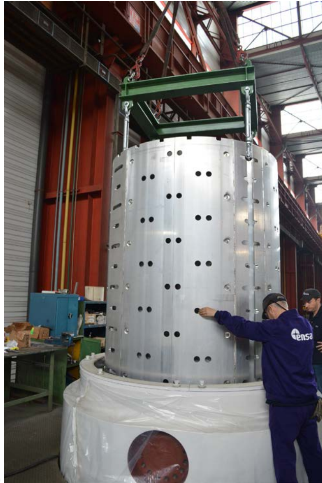
Figure 3-3. ENUN 32P cask basket (a) and its insertion into cask (b).
