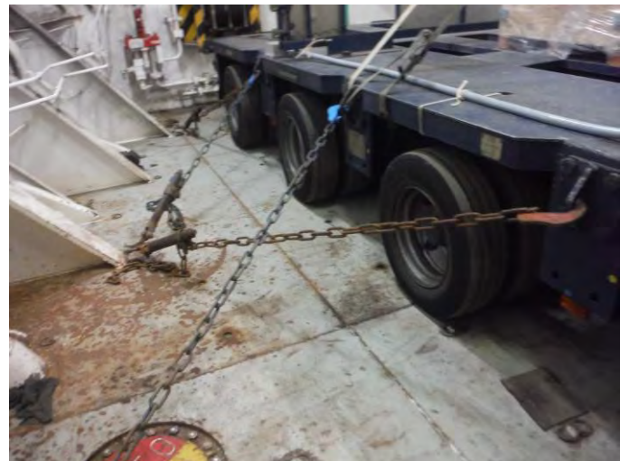
10. Lashing from platform to deck
