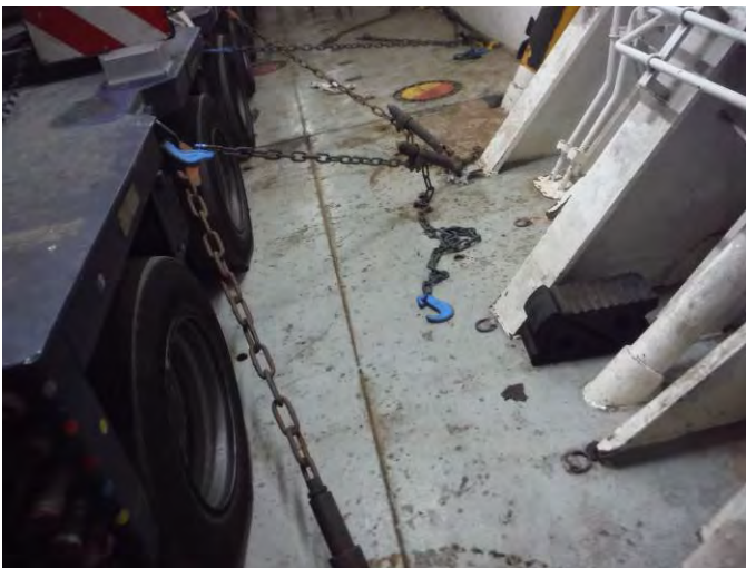
9. Lashing from platform to deck
