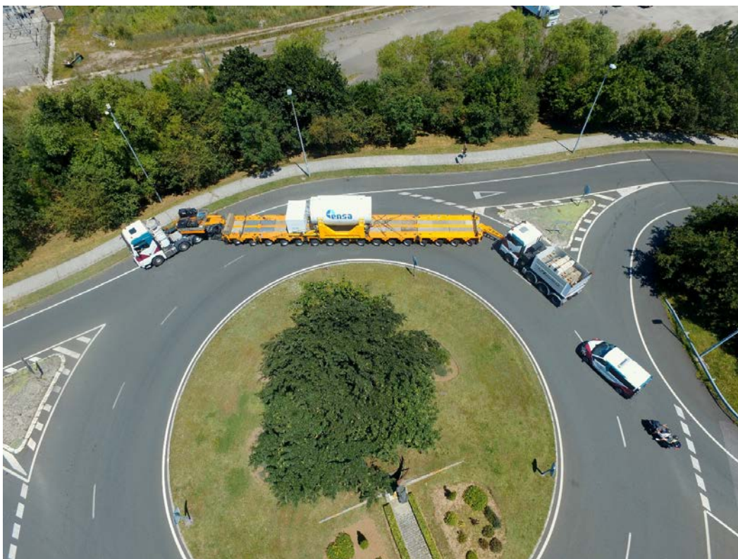
Figure 4-16. Heavy-haul truck negotiating one of the ubiquitous roundabouts. Note length of the 17-axis trailer mandated for this transport by the Spanish Ministry of Public Works and Transport.
