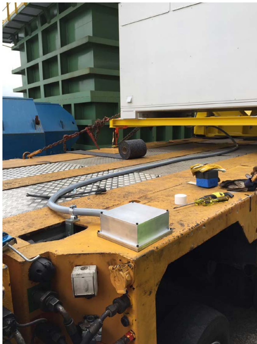
Figure 4-11. Triaxial accelerometer enclosure on Heavy-Haul Truck Trailer.
