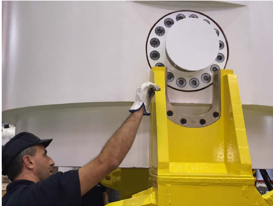
Figure 3-37. Cask being set on cradle.
