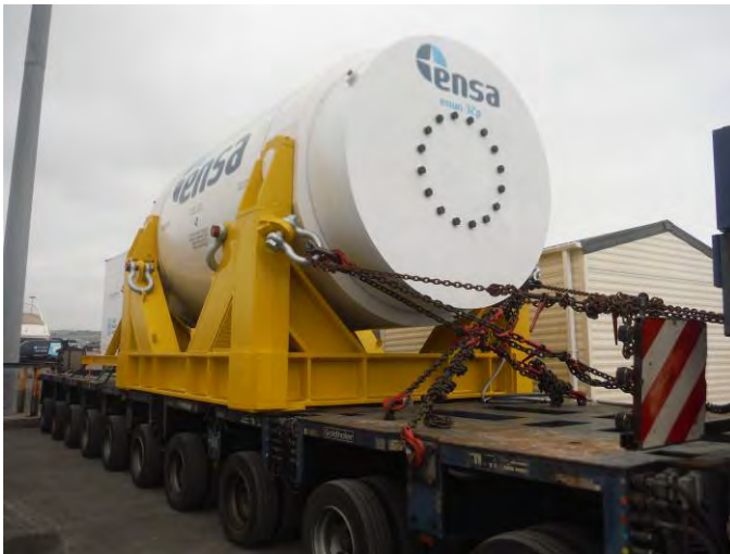
1. Lashing with chains in fore part
