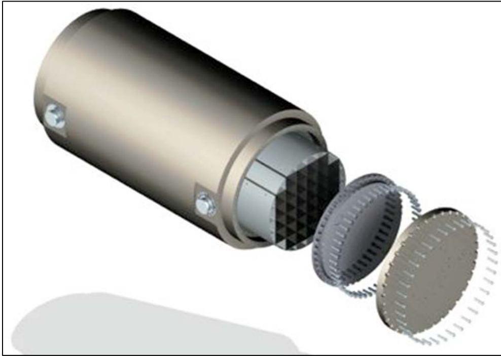
Figure 3-5. Illustration of the two lids of the ENSA ENUN 32P cask, which were replaced with an instrumentation test lid for the tests.
