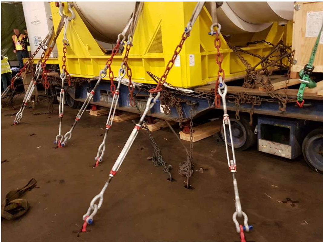
Image 13. SAMSON and CASK on board of MV Tarago, lashed and secured to vessel deck.
