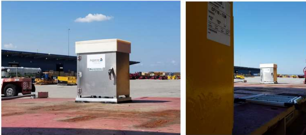
Image 13. GPS system completely installed at “A end” of railcar. July /21 st
