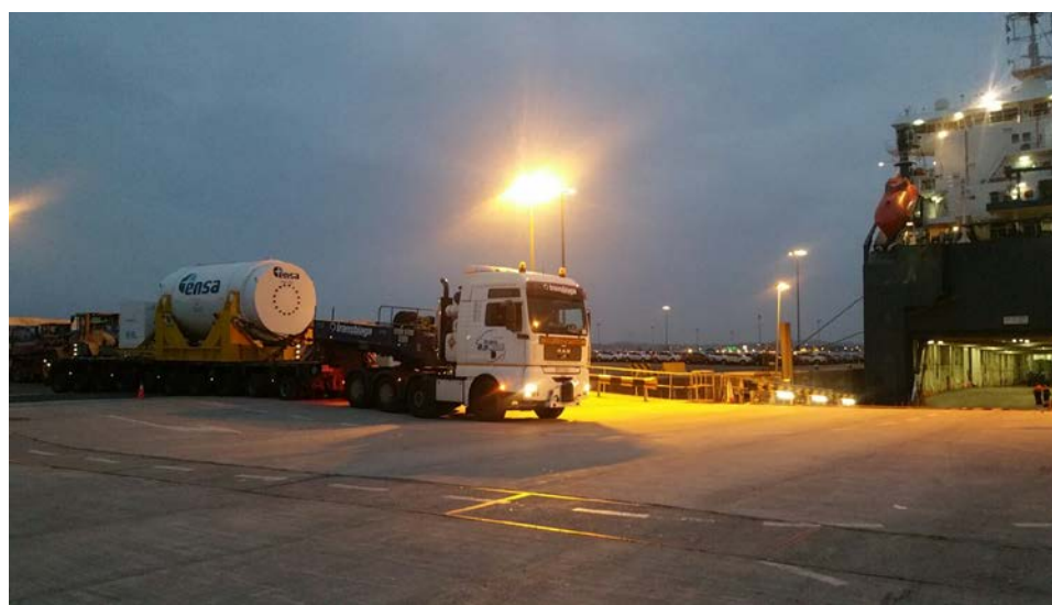
Figure 4-24. 10-axle truck trailer used for Roll-on/Roll-off ship transport from Santander to Zeebrugge.
