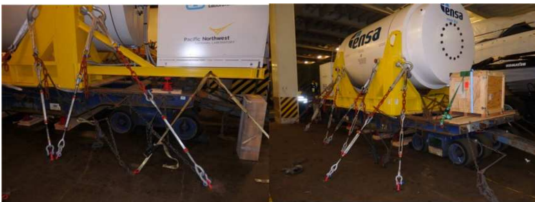
Typical lashing between cradle and deck
