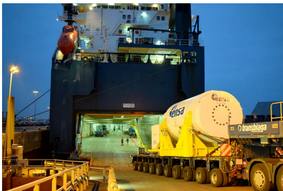
Figure 4-26. Cask entering the Ro/Ro ship “Autosky” at the Port of Santander.
