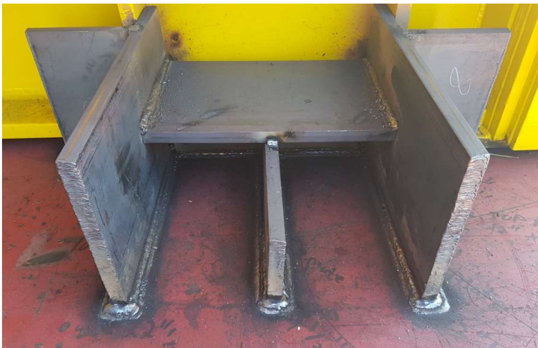
Image 16. Picture of final configuration of one complete stopper composed of several plates. 2 (4 complete stoppers like image 16 were welded in total, 2 at both sides of CASK.).
