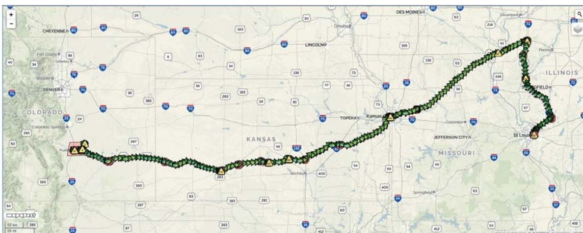
Figure 4-54. Route of 18-day data collection (bottom) as recorded by Lat-Lon GPS unit mounted on cask.
