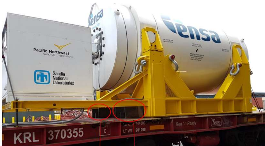
Image 17. 2x stoppers in the back side of CASK.
