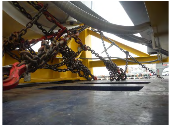
2. Lashing with chains in aft part
