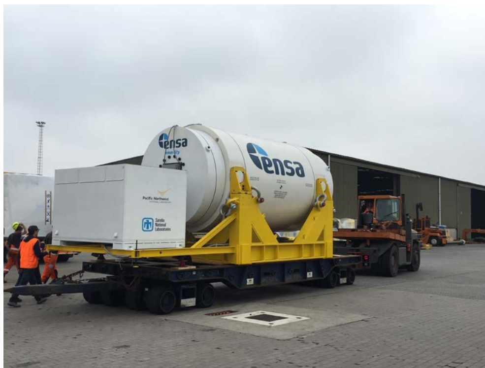
Figure 4-32. Cask system being moved on Samson to dock.
