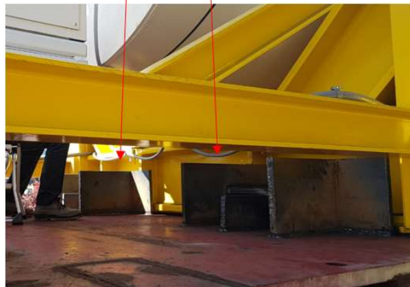
Image 18. 2x stoppers in the front side of CASK
