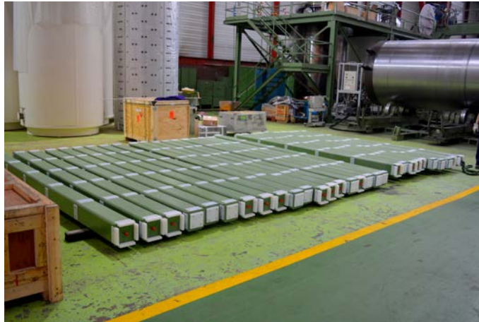
Figure 3-31. Twenty-nine dummy steel and concrete assemblies used to simulate the weight of actual fuel assemblies.
