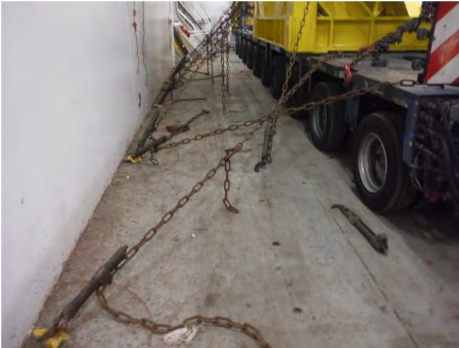
7. Lashing from platform to deck
