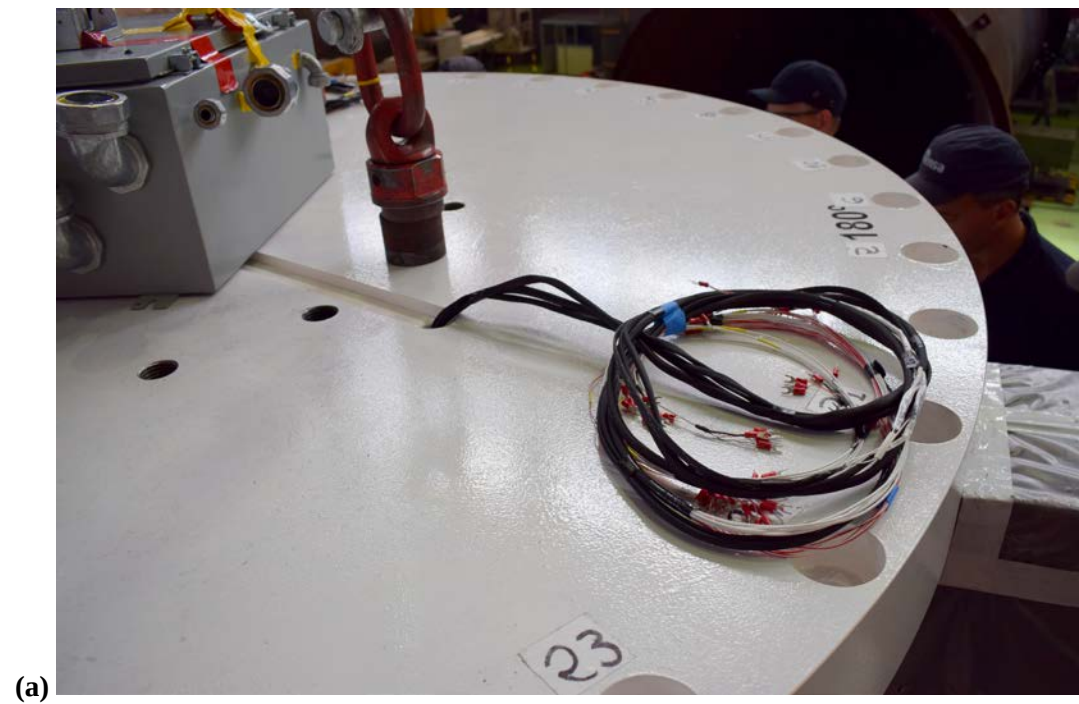
Figure 3-7. Placing the instrumentation lid on the cask.
