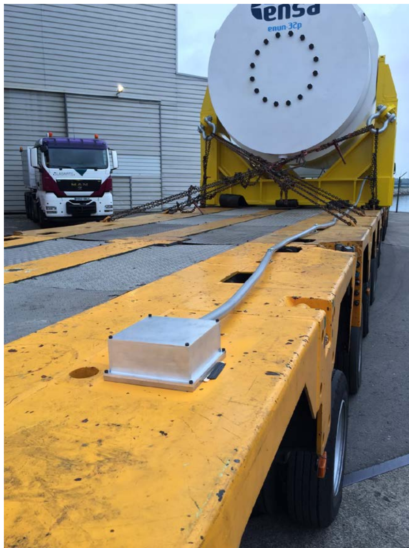
Figure 4-10. Triaxial accelerometer enclosure on Heavy-Haul Truck Trailer.
