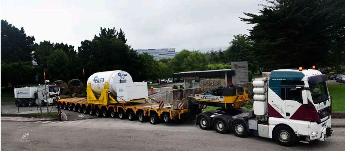
Figure 4-12. Cask system departing ENSA for Heavy-Haul Truck Test.
