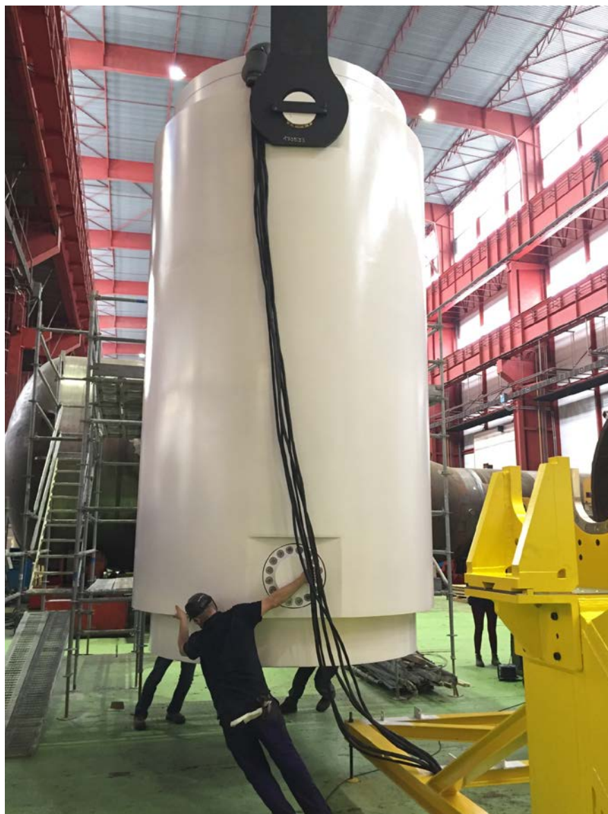
Figure 4-3. Positioning cask for Cask Handling Test.
