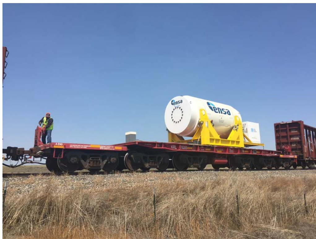
Figure 4-39. Kasgro 12-axle railcar used for transport of cask unit from Port of Baltimore to the TTCI near Pueblo, Colorado. Note the ANL Traveler GPS unit in the white-topped gray box and the Data Acquisition/Battery Box to the right of the cask.
