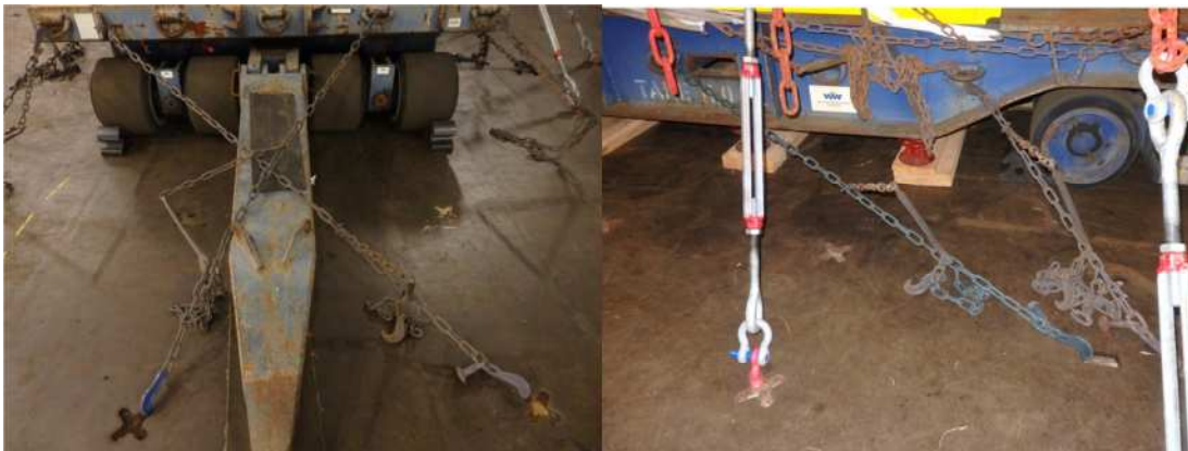
Typical lashing between SAMSON and deck
