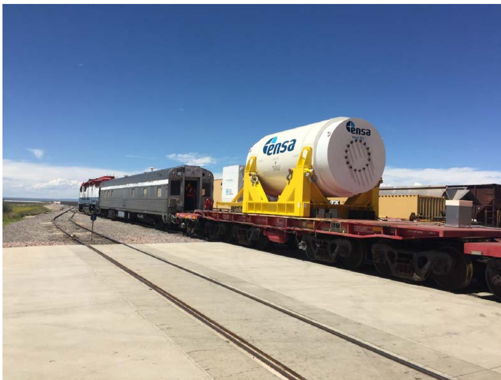
Figure 4-48. Cask system on the Kasgro 12-axle railcar. The gray car between the locomotive and cask railcar is the TTCI Instrumentation Car where TTCI and SNL technicians were located during the rail tests.
