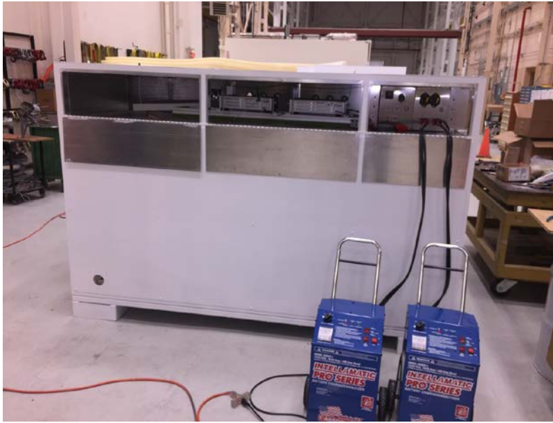
Figure 3-29. Data Acquisition/Battery Box. Siemens LMS SCADAC 5-slot Recorders with LMS SCADAC Mobile 8-channel universal durability input modules and battery chargers shown
