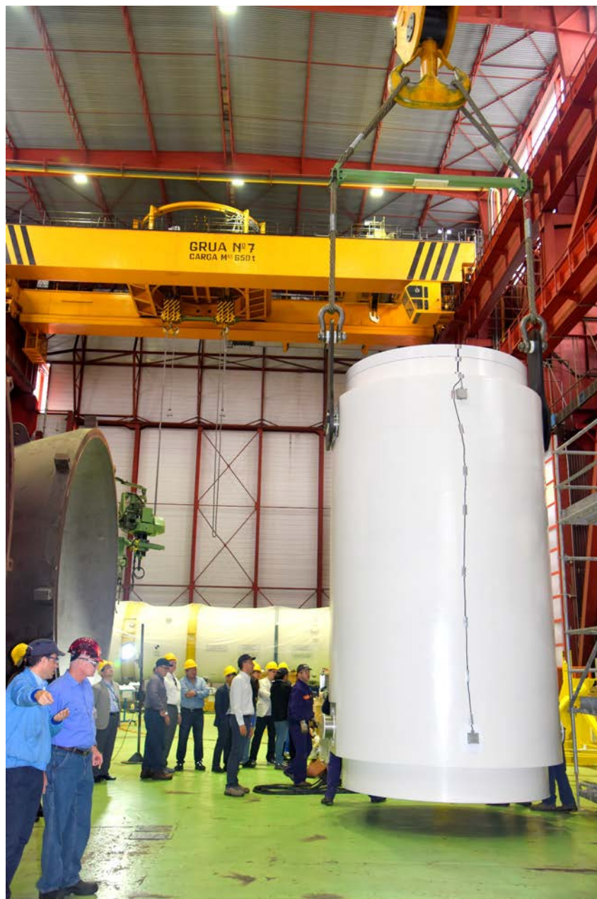
Figure 4-4. Cask Handling Test.
