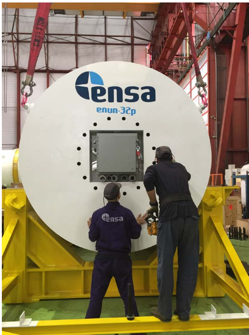
Figure 3-39. Top impact limiter g placed on instrumentation lid. An opening had been machined into the limiter to accommodate the Junction Box.
