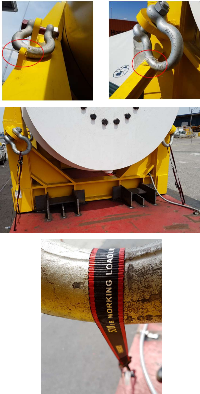
Image 12. Shackles were fixed by straps to the cradle or textile slings to the railcar to minimize any background noise caused during the railway transport that may affect the data.
