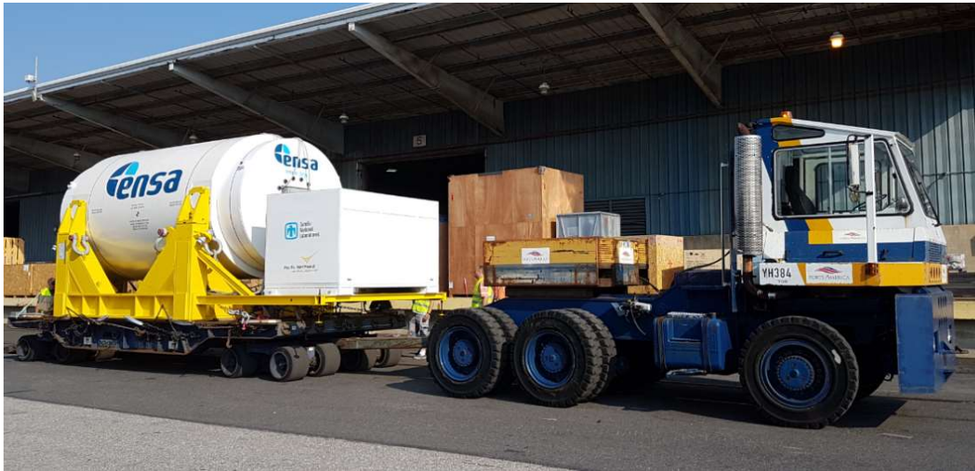
Image 1. Cask on SAMSON with tug master about to be moved next to crane for transshipment from SAMSON to RAILCAR at Mid-Atlantic Terminal. July/19 th
