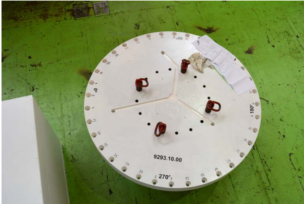
Figure 3-10. Cask test lid. Note the three holes at the end of the recesses machined into the lid. The holes provided the exit path for the instrumentation cables, which were laid into the recesses to the circular region in the middle of the lid from which the cables entered the Junction Box.
