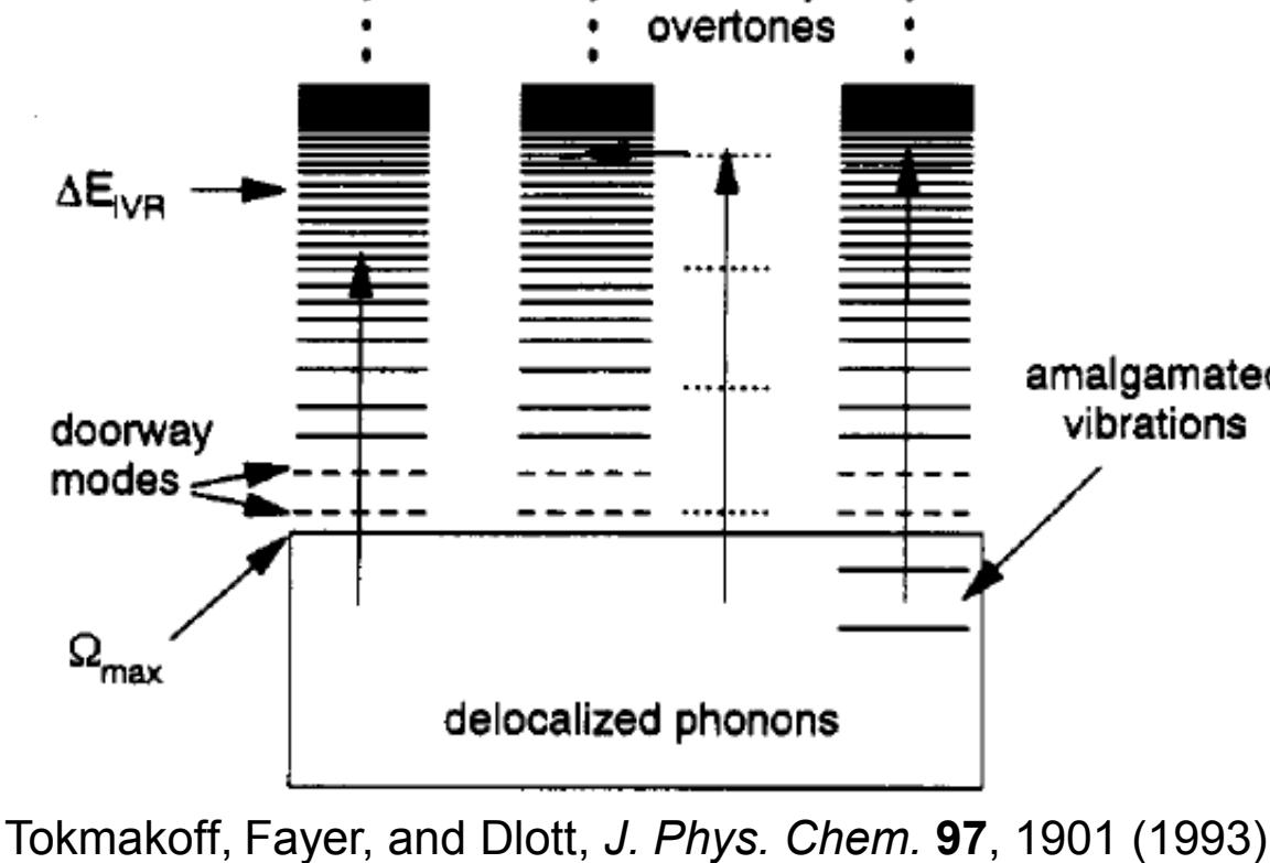
Several pathways allow for energy transfer between low-frequency phonons and high-frequency molecular vibrations. Low-frequency "doorway" modes are key. Anharmonic coupling couples the molecular vibrations with phonon modes of crystal:
