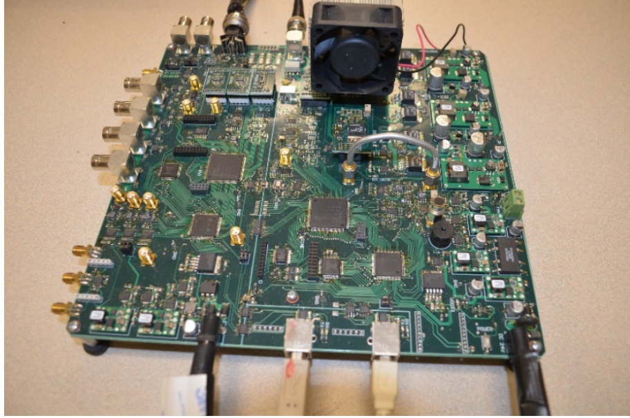
Fig. 6: Circuit board which includes an add-on circuit for use with the Zurich lock-in amplifier on the left side of the circuit board and on the right a prototype an alternating current potential drop (ACPD) measurement circuit. At the top of the picture, the large object is a heat sink for a trans-conductance amplifier (TCA) which provides a predefined current to the probe at frequencies below 10 kHz. A smaller TCA provide current at frequencies from 10 kHz to 100 kHz.
