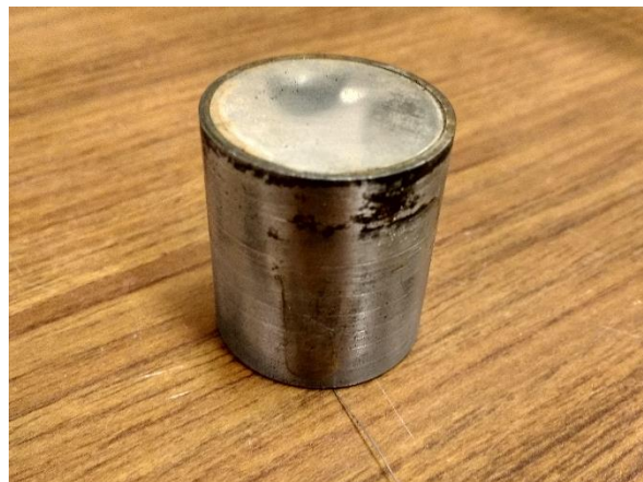
Figure 6.6 Rust developed on the Ultrasonic transducer after third heating cycle due to the oxidative reaction of low carbon steel casing with water
