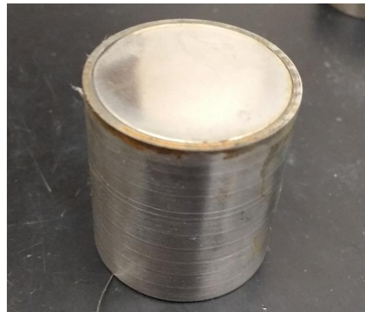
b) Rust developed due to oxidative reaction of low carbon of steel with water
