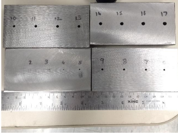
Figure 7.2 Side drilled holes with diameter varying from 0.46mm to 3.9 mm in a 1018 low carbon steel block
