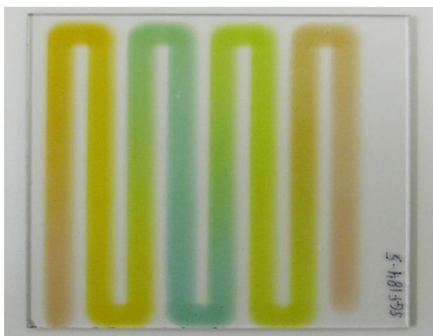
Figure 4. A spray coated film of dye-loaded PEG demonstrating five primary colors along the spray line (Red-Yellow-Blue-Yellow-Red). This demonstrates the ability of the instrument to control composition along a spray line with multiple source solutions.
