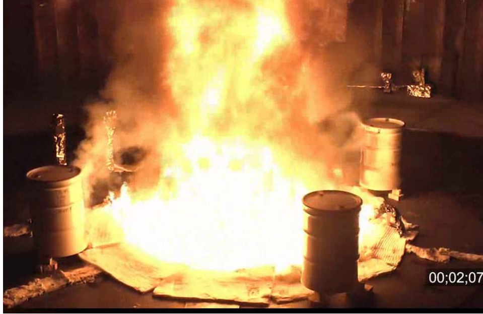
Figure 4-2. Four 55-gallon drums containing assorted trash on the circumference of a three-meter pool fire.
