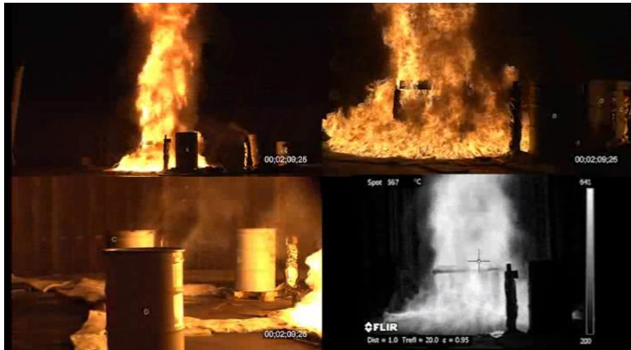
Figure 6. Image of an indoor POC fire test showing fully engulfing conditions of the center POC drum, and showing the surrounding POC drums (bottom left).
