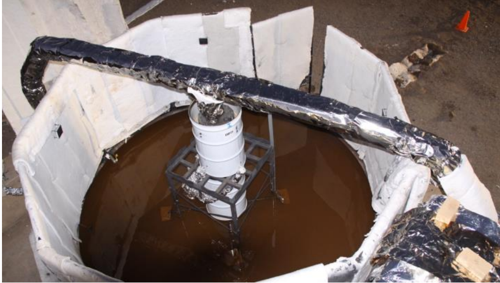
Figure 7. Image of the POC drum inside the outdoor test cell. Note that there is no drum lid, and plastic liner, Celotex, and wood board cover in the top drum.
