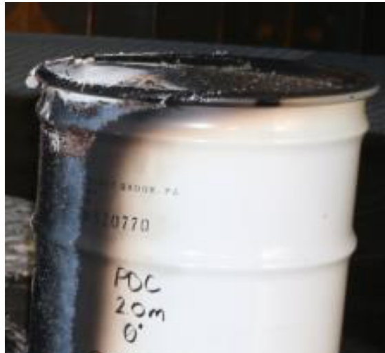
Figure 11. Bulging of the 7A drum lid on a POC at 2m from the center of the fire.
