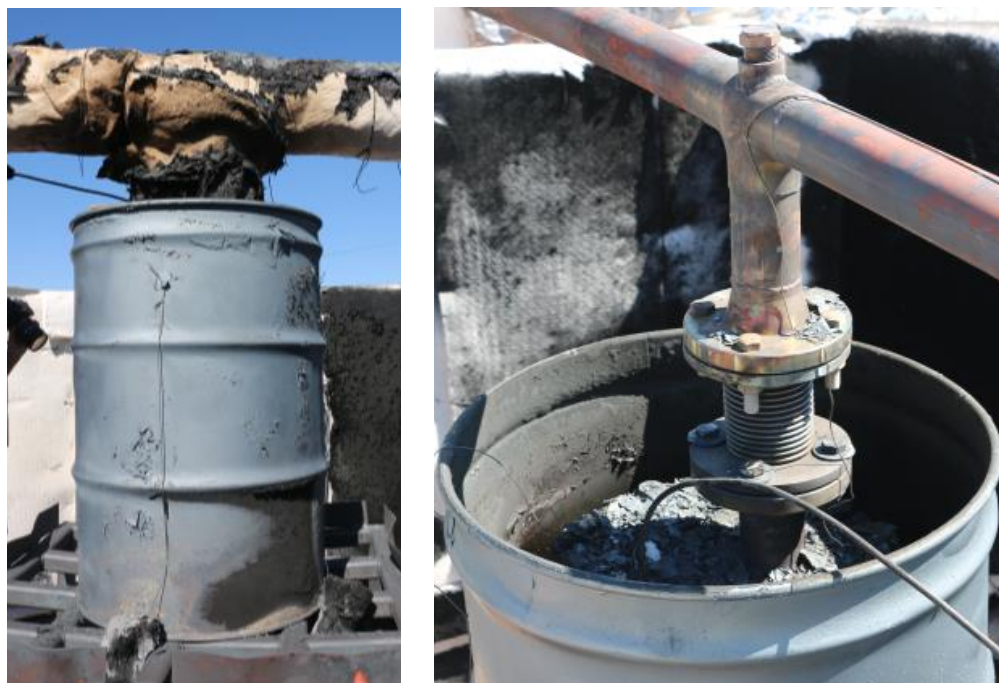
Figure 14. POC drum without a lid after the 30-minute engulfing fire. The right image shows a close-up of the vertical section of the pipe after the test when the insulation was removed. The bellows portion of the vertical pipe was added to allow for unobstructed deformation of the PC lid due to thermal stresses.
