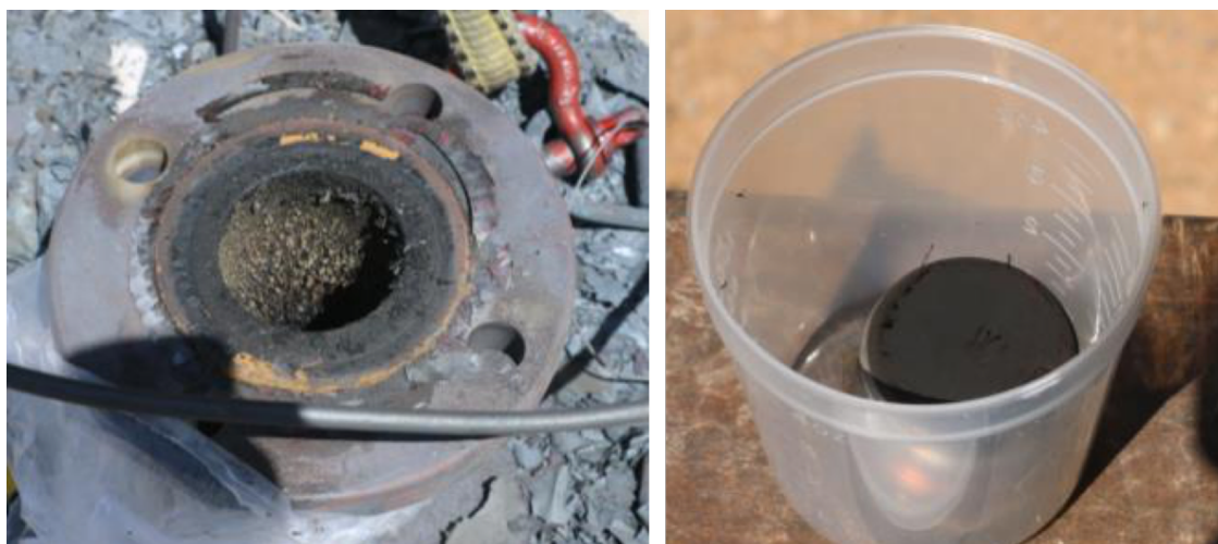
Figure 15. Material collected on the first section of the vertical pipe (left) and on one of the sample coupons on the horizontal section of the U-shaped pipe (right).
