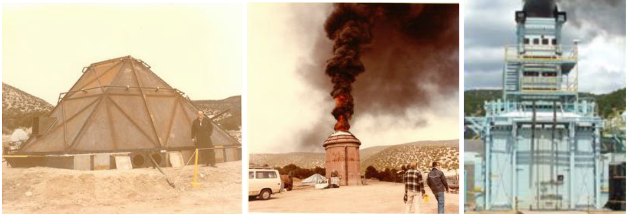
Figure 2. Left, the SWISH, a water-cooled wall enclosed pool fire facility for a 1 x 1 m pool. Center, the LAARC insulated wall enclosure for a 3 m dia pool fire with passive air control. Left, the SMERF, a water-cooled wall enclosure for a 3m x 3m pool with active air control.
