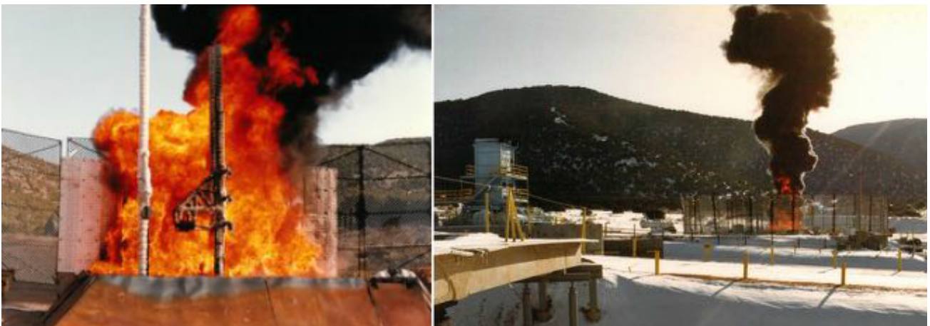
Figure 3. The 6 m x 6 m outdoor pool with 6 m high wind fences. The fences are located at a distance from the pool edge.
