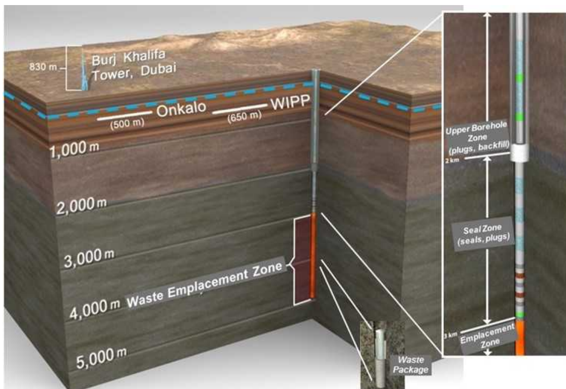
Fig. 1. Generalized schematic of the deep borehole disposal concept.
