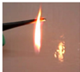
Commercial separator after exposure to fire
