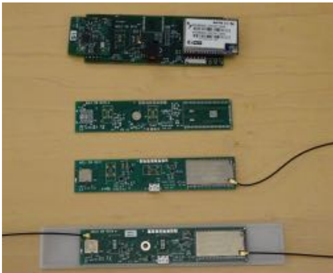
Figure 3: MoJo Bridge PCB Prototypes, with final PCB Prototype on bottom in plastics.
