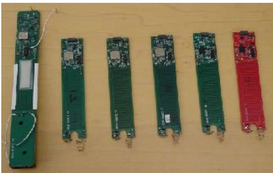
Figure 1: Remote PCB development progression with final pre-production Remote PCB on right.
