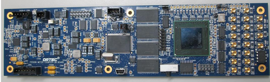
Figure 2 Photograph of the List-Mode Fission Meter Board installed into the Fission Meter for the MC-2014 Measurement Campaign
