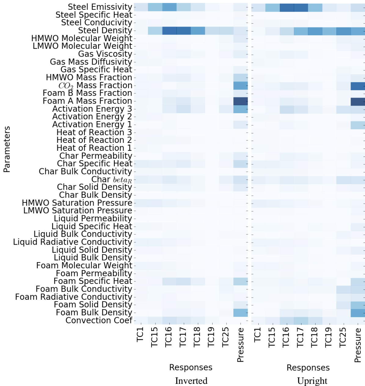
Figure 81: Heat maps that correlates each parameter with each response for the inverted (left) and upright (right) simulation. A darker color indicates that the response is more sensitive to the parameter. In this map, 'Heat Flux' was removed at a parameter in order to be able to view the effects of the other parameters.
