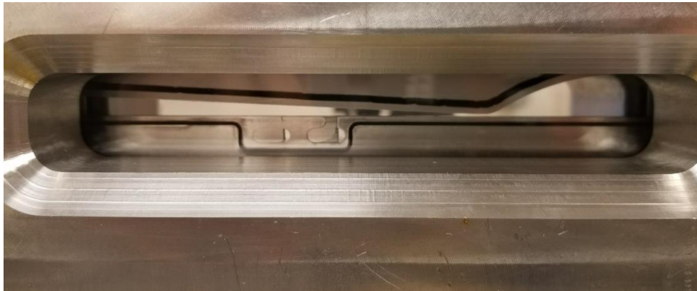
Figure 24: New converging-diverging nozzle profile fabricated and installed in the venturi test section. The new C-D profile lowers the mass flowrate requirement by a factor of 2, increasing the range of operating conditions that can be investigated.
