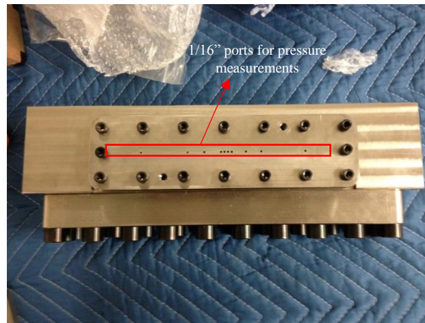
Figure 16: Assembled test section showing the static pressure ports
