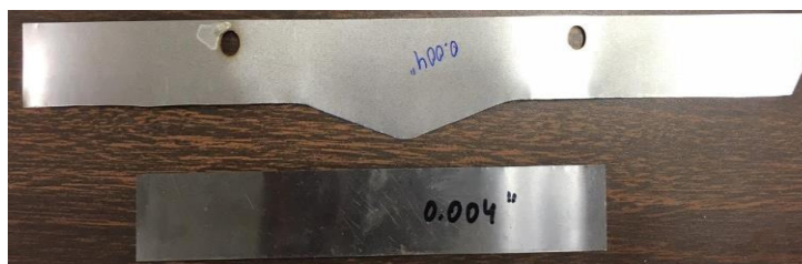
Figure 20: 316 stainless steel shim stocks cut in shape of the venturi profile
