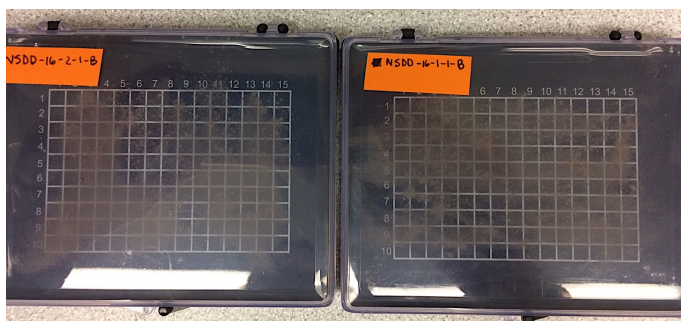
Figure 3. Images of the sample-loaded Gel Pak boxes used for obtaining autoradiographs of the two samples provided to LLNL. Grids are 8.5 x 5.5 cm.
