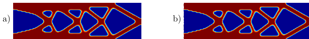
Figure 8: The optimized designs for the 1kN load for a) the secant cost and b) tangent cost functions.
