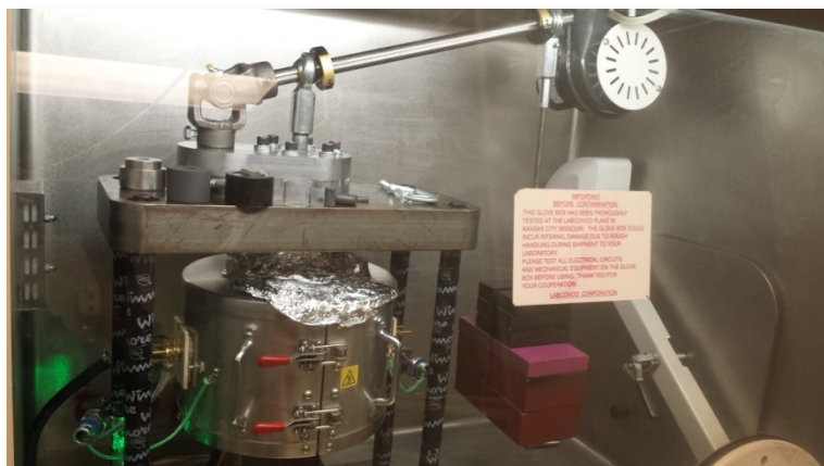
Figure 4: Hot Uniaxial Press implemented in a standard size glove box operating at 770 °C and 75 MPa under argon. The lead weights (right) are marked and calibrated for pressure in regard to the current level settings
