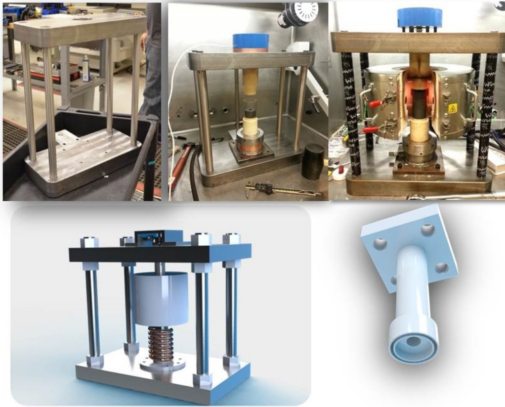
Figure 2: Mark I design of a remote operated radiological uniaxial press (ROHUP) together with the Solid Works drawing.
