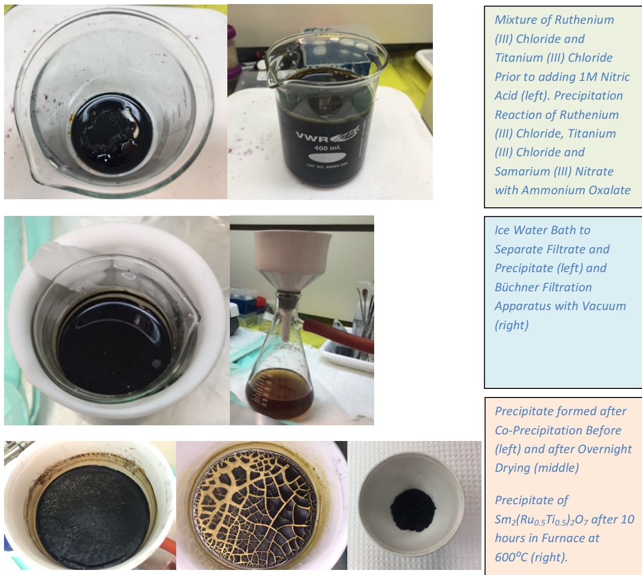
Figure 23: Illustration of crucial steps of Co-Precipitation of \text{Sm}_2(\text{Ru}_{0.5}\text{Ti}_{0.5})_2\text{O}_7
