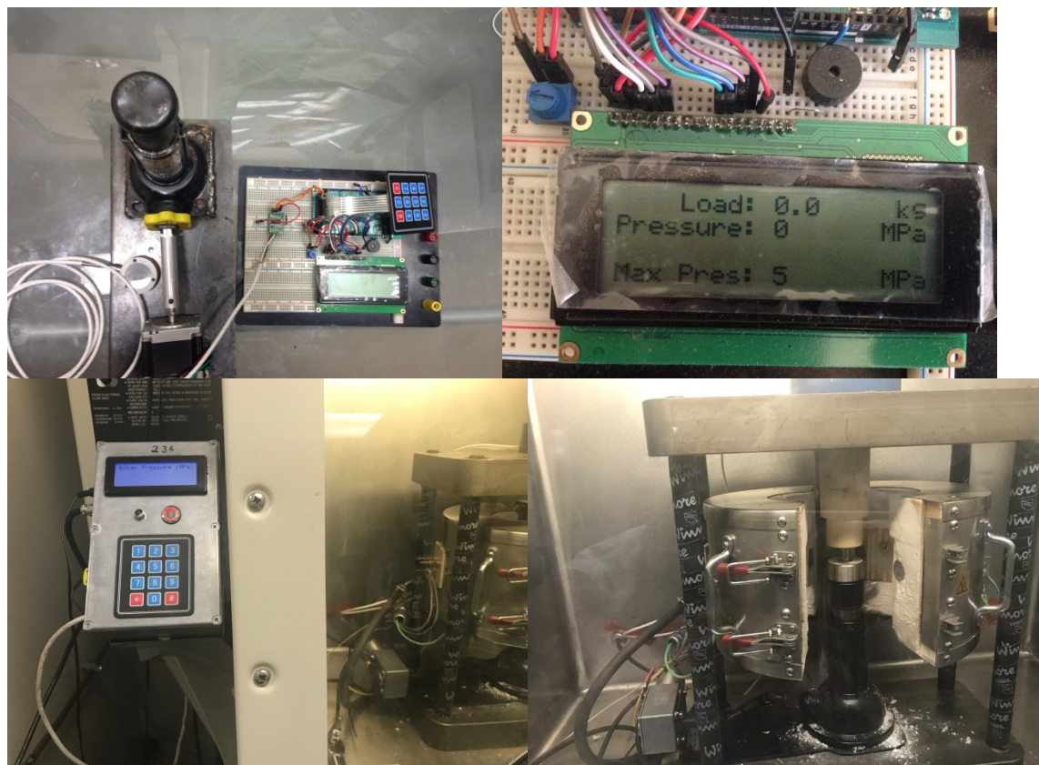
Figure 6: Mark III uniaxial hot press design applying an electro-mechanical load system and a hard-wired controller. The hot press is located in a radiological atmosphere controlled glove box.
