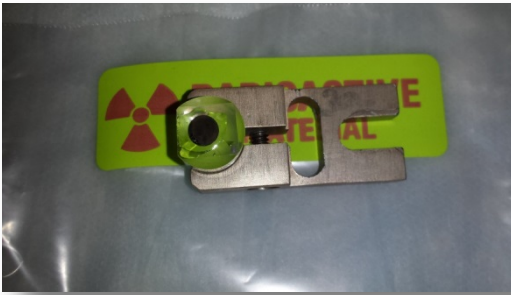
Figure 41: Preparation of hot-pressed \text{SrTcO}_3 perovskite (SPE1) test specimens for ASTM C1220-10 leaching experiments for 28 days
