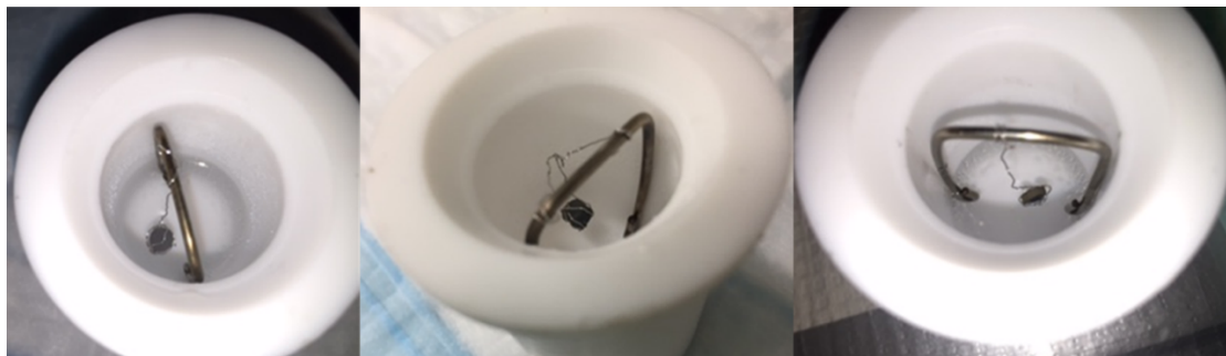
Figure 48: Pellets in Leachate in PTFE Vessels after corrosion test. No visible solids were seen the leachate.
