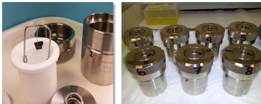
Figure 34: Stainless steel sample hanger with glass specimen (left), Parr 23 mL 4749 digestion vessels (right).
