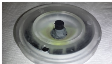
Figure 10: HUP produced monolithic “ \text{Sr}_2\text{TcO}_4 ” pellet (10 days at 570 °C and 80 MPa), before (top) and after (bottom) XRD analysis. The pellet lost its physical integrity during the 2 hours of XRD analysis due to swelling and potentially the formation of strontium hydroxide.
