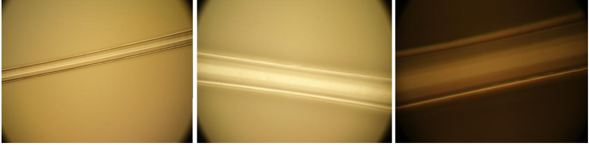
Figure 86: Photos of the sapphire fiber that was heated in an inert atmosphere at 4x (Left), 10x (Center), and 40x (Right) magnification.
