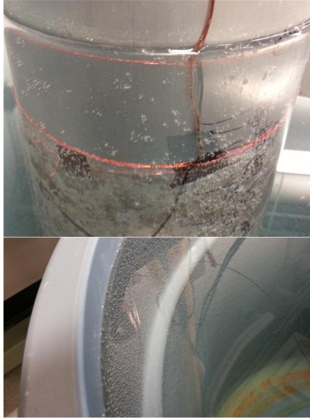
Figure 51: Pictures of the dry tube instrumented with a K-type thermocouple and the dissolved oxygen coming out of solution at the surface of the dry tube and the trash can.
