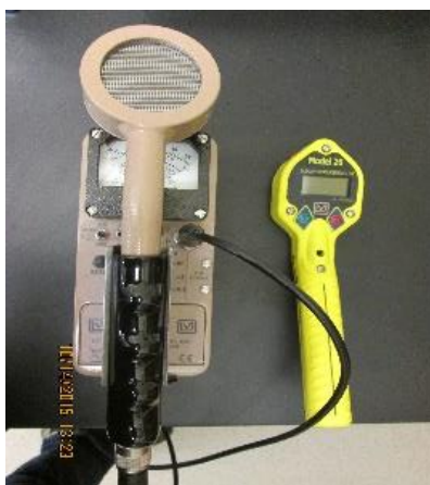
Figure 3.3 Pancake detector frisking meter (left) and hand survey meter (right) from Atlantic Nuclear Corporation.
