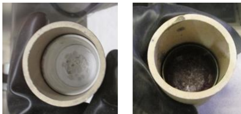
Figure 3.9 Alumina crucible (left) and Inconel crucible (right) placed in safety crucible for preliminary and uranium studies, respectively.
