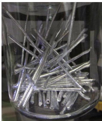
Figure 4.17 Purified Cd rods under argon environment.
