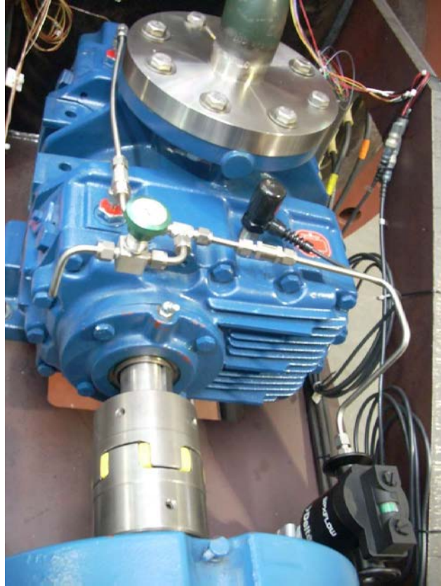
Figure 17 - Installed pressure relief system to relieve pressure from the blower gear boxes.
