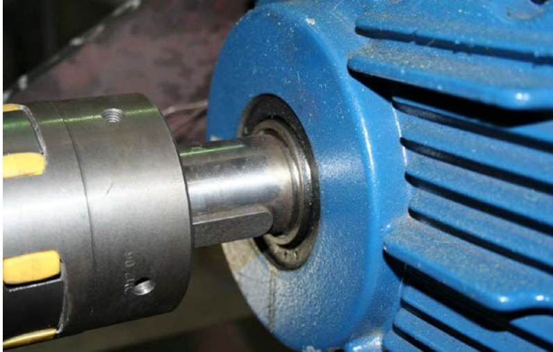
Figure 1 – Oil drip trace at the shaft seal of the blower.
