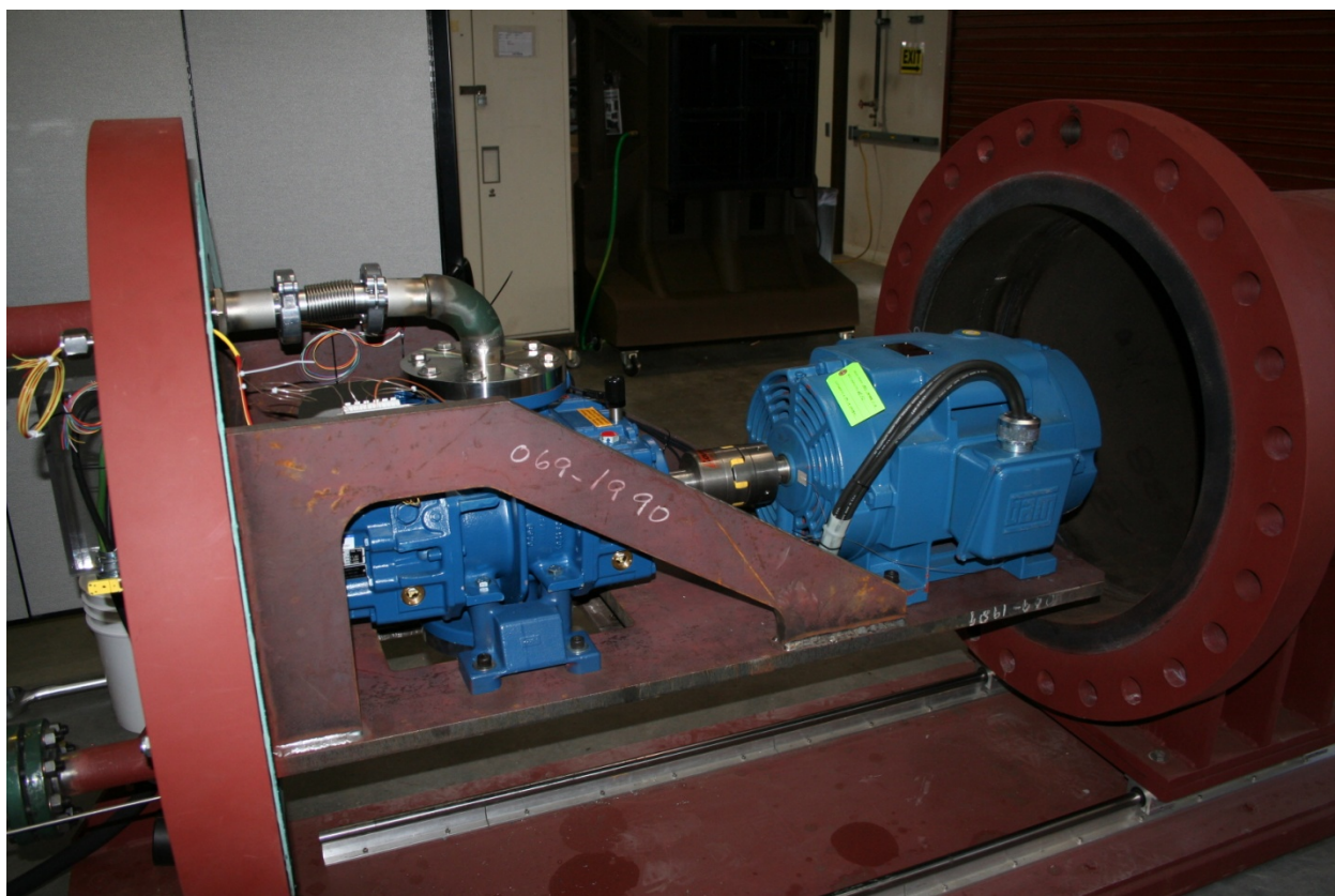
Figure A4. Close-up view of the blower, on the left, with motor. Motor is wired and blower exit piping is installed. (top left).
