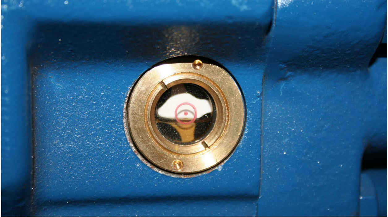
Figure 9. Oil level sight glass, showing some loss.
