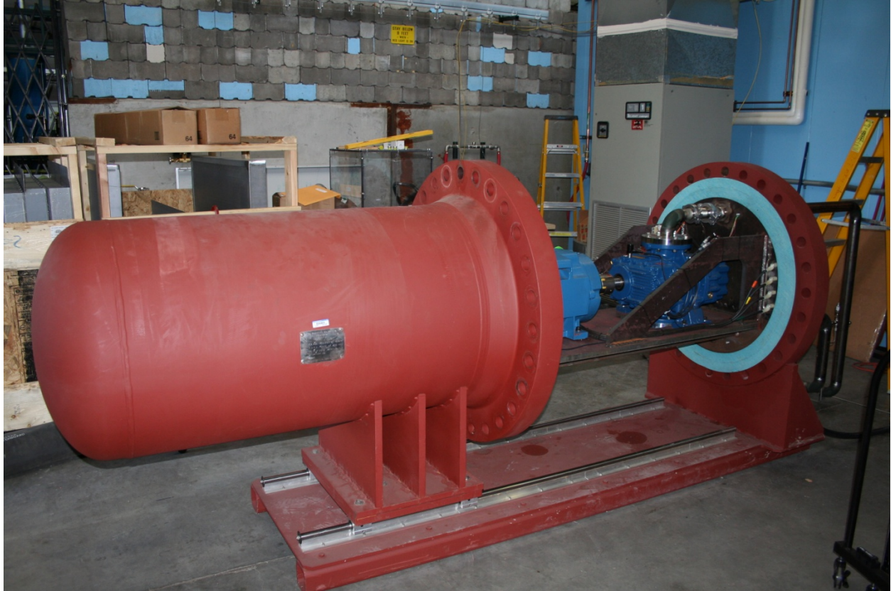
Figure A3. Vessel open, showing blower and motor.
