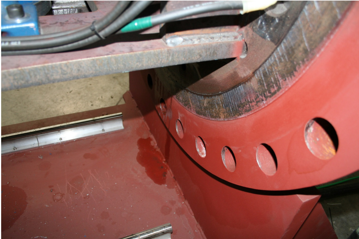
Figure 11. Oil on the vessel bulkhead, and dripping to the platform below after opening the tank.
