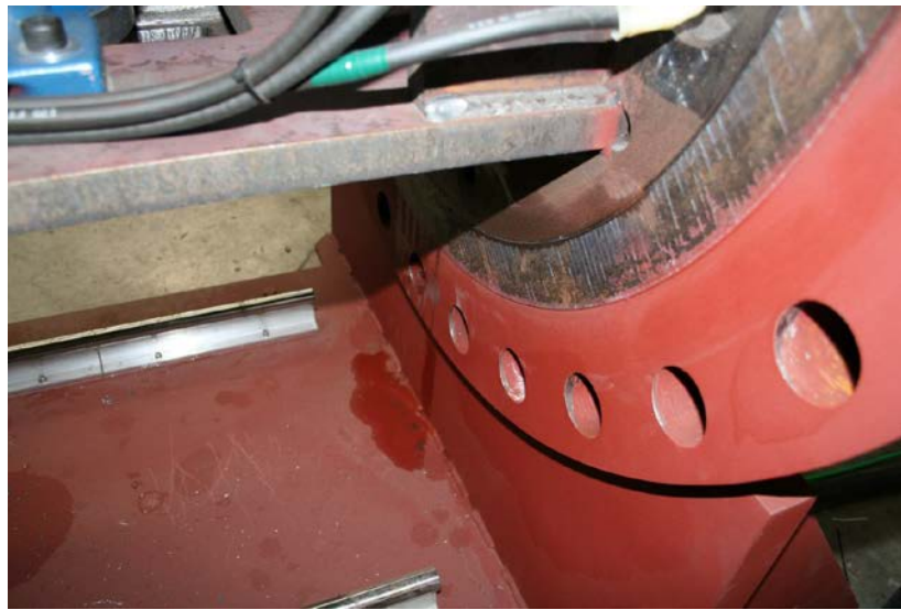
Figure 2 - Oil on the vessel bulkhead, and dripping to the platform below after opening the tank.
