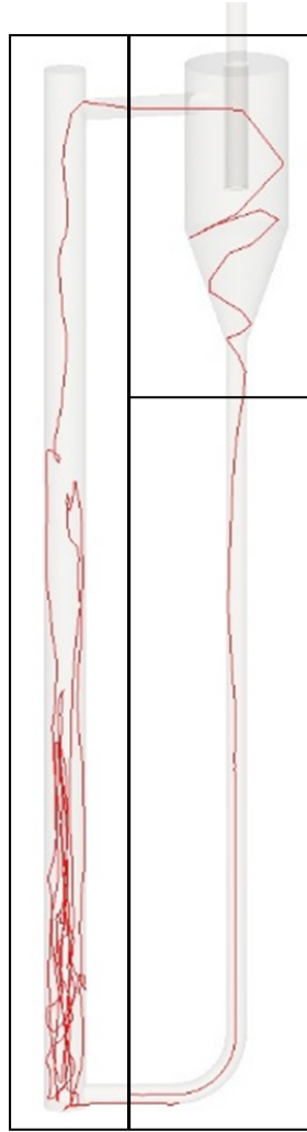
Figure 11: Trajectory of a tracer particle inside the CFB and the division of the system for the calculation of the residence times.
