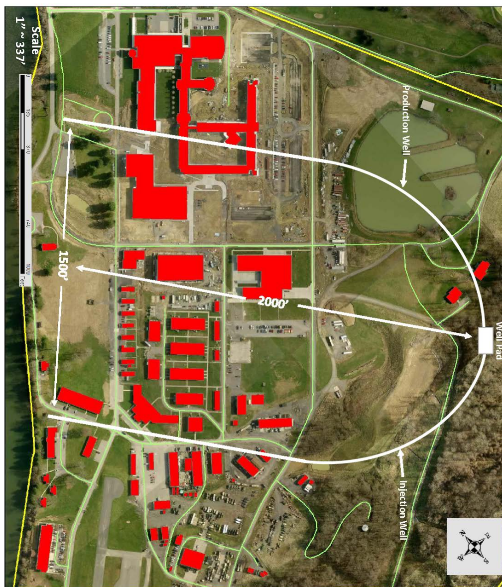
Figure 42: Plan view of proposed horizontal wells for geothermal heat capture. (Map of buildings provided by Camp Dawson)
