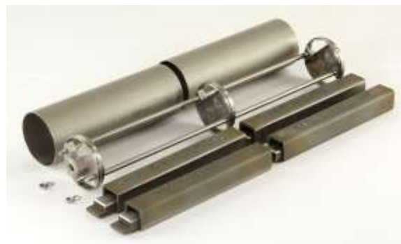
Figure 2-13 Creep test sample fixture. The samples are sandwiched between two curved plates that are tightly fitted into the rectangular holder.
