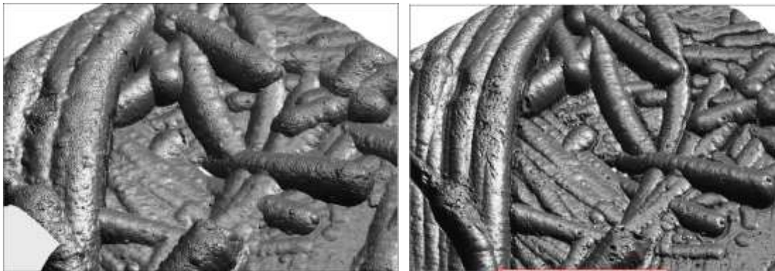
Figure 2-16 – Surface fiber CVD coating diameter change.
