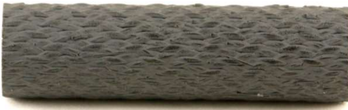
Figure 2-18 – Tubing sample exposed to heavily hydrogenated PWR water chemistry. Measurement showed no weight loss.
