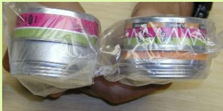
Figure 1. A comparison of non-certified (on the left) and certified (on the right) respirator cartridges. Note that they are similar in size and appearance.
