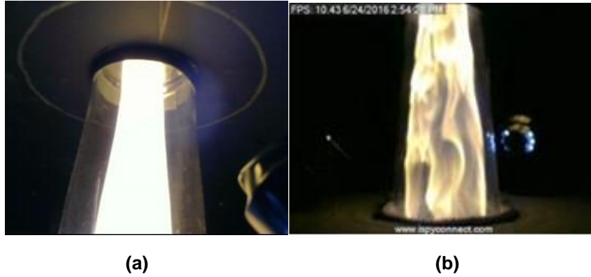
Figure 6-4. Photographs from initial firing tests in the 100kW POC facility.(a) laminar and (b) turbulent methane/air flames. The quartz reactor wall can be easily observed in (a).
