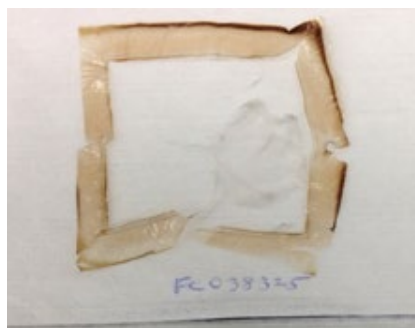
Figure 106. Image of the three membrane MEA after separating layers. A section of the fully separated 725EW PFSA center layer can be seen in the center/right section.
