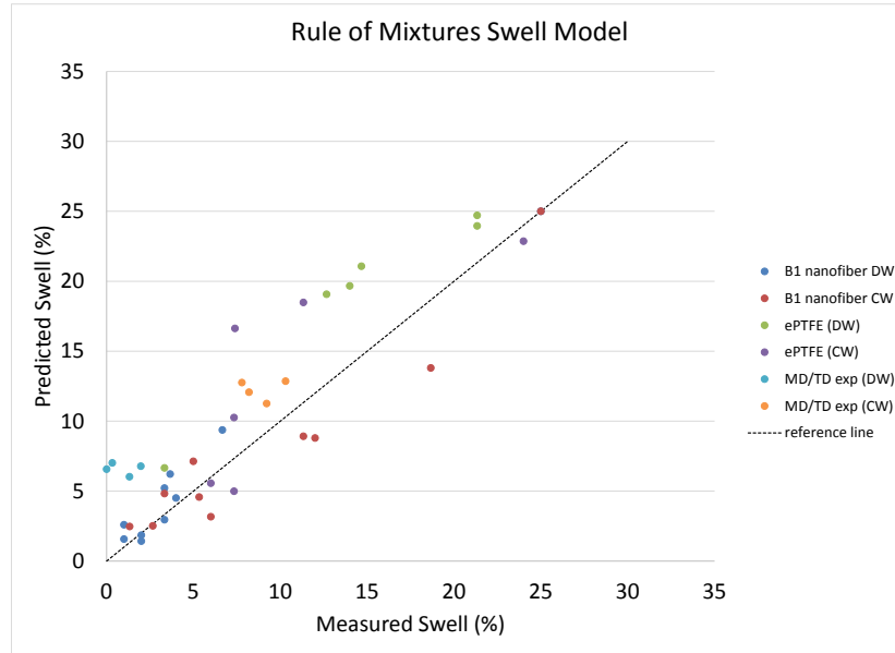
Figure 59. Comparison between measured swell data and predicted data based on rule of mixing model. Reference line represents the ideal case (45° line) and not a curve fit.
