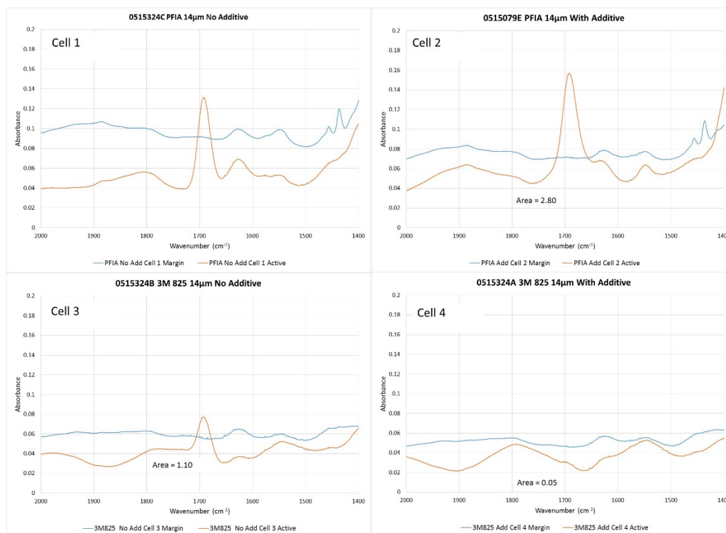
Figure 71. FTIR spectra of K + - exchanged membranes after H 2 O 2 vapor degradation.
