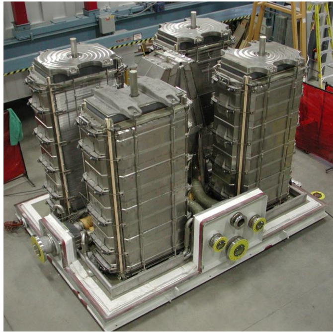
Figure 1-3. Fuel Cell Module with Module Enclosure Removed
