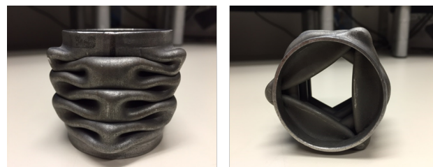
Fig. 5. Tubular crush box impact limiter, after crushing (Ref. 3; photos provided by Brad Day, SNL).
