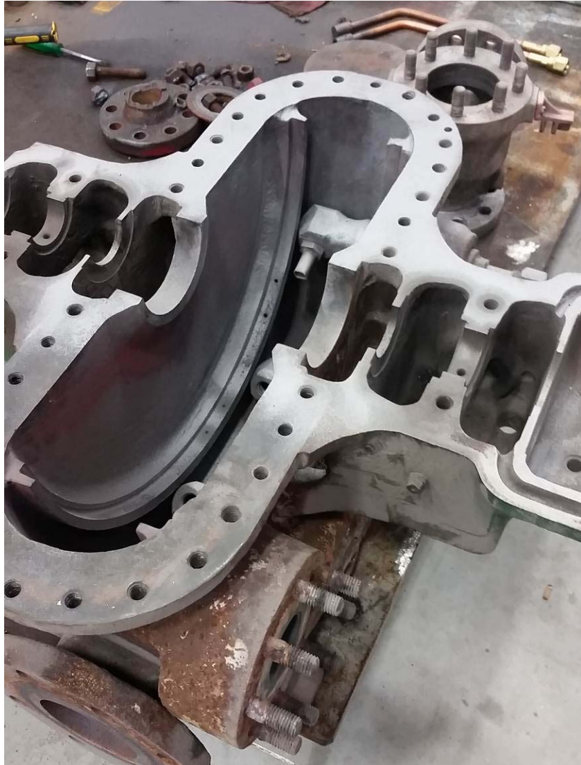
Figure 40 Lower casing, after sandblasting, with two nozzles removed
