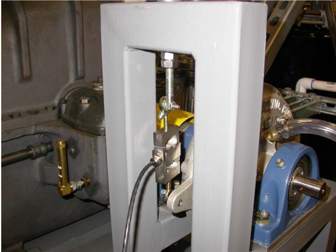
Figure 60 Load cell attachment to dynamometer
