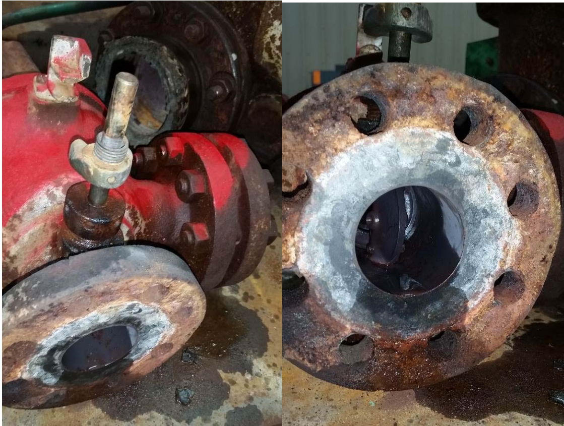
Figure 38 Trip Throttle Valve, with seized valve stem
