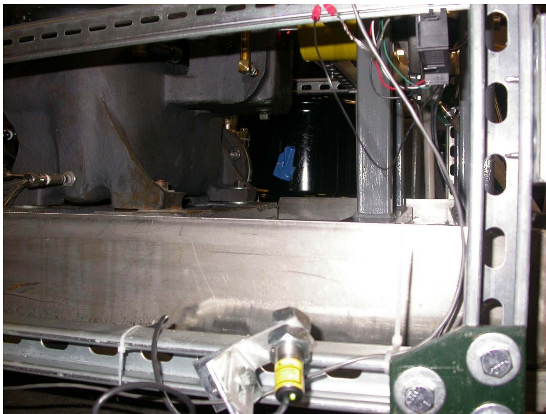
Figure 57 Monarch ROLS-W Tachometer sensor
