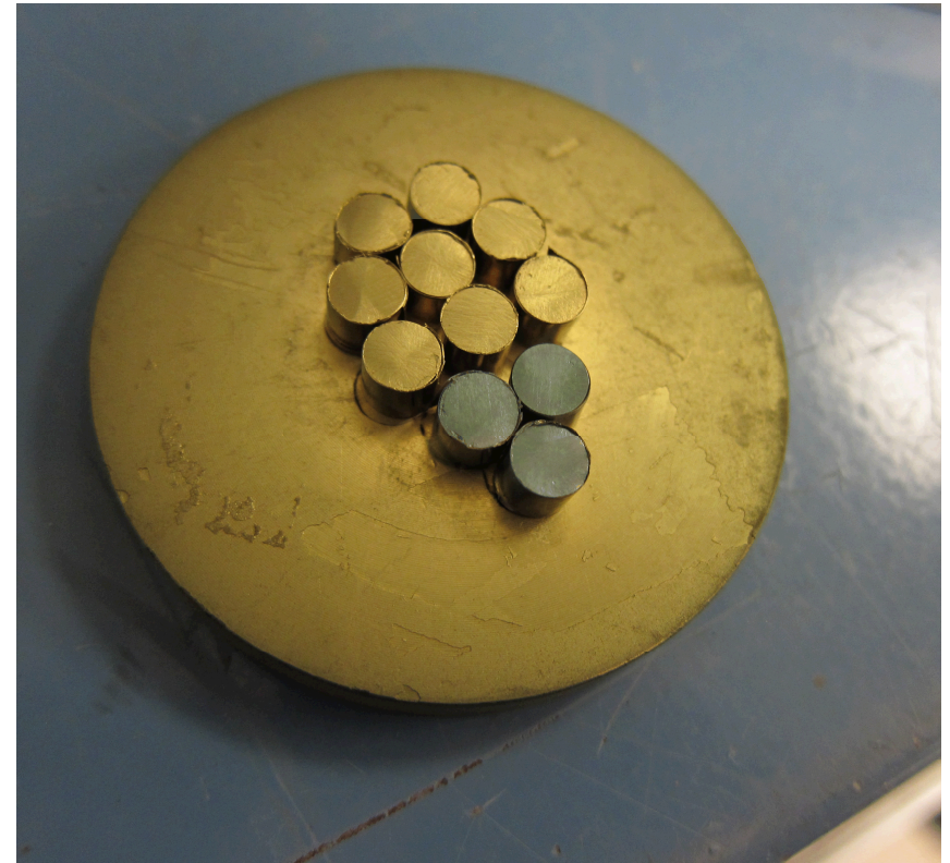
Electroding 1/4" sintered pellets in preparation for I-V testing
