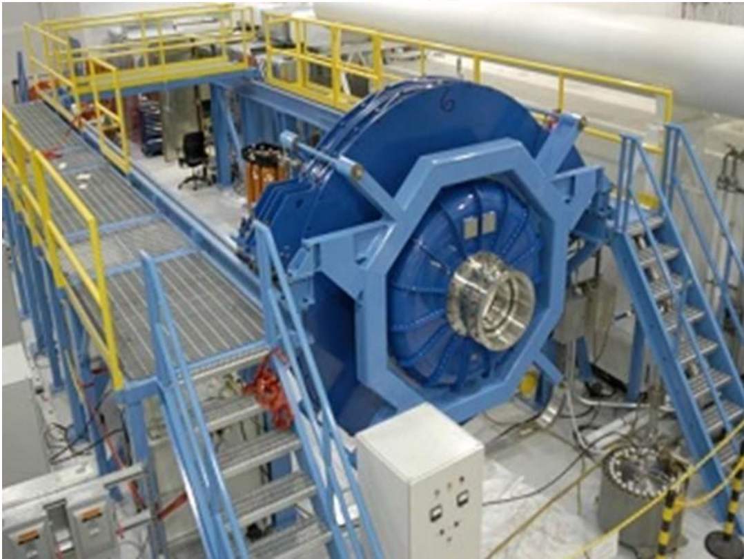
Figure 22. Illustration of the 1 MV, 1 MA MYKONOS pulsed power facility at Sandia.
