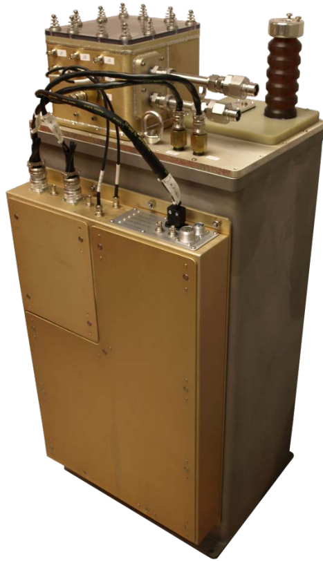
Figure 46. Thyatron replacement switch (as built)
