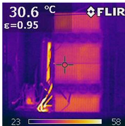
Figure 41. Thermal image showing uniform current distribution in the switch circuit boards stacked two high.
