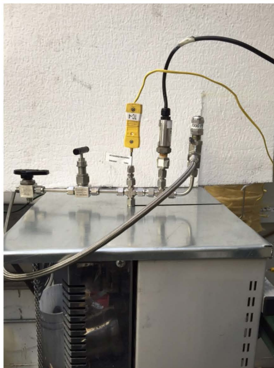
Figure 4-16. Photograph of valves and instrumentation hookups above the clamshell heater. Left to right: fill valve, needle valve, thermocouple, pressure transducer, pressure relief valve. Photo reproduced with permission from University of North Dakota EERC.
