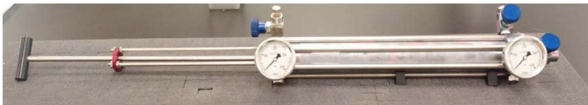
Figure 4-8. Representative ASTM D8009 manual syringe sampling cylinder. Reproduced with permission from Bagawandoss (2015a).
