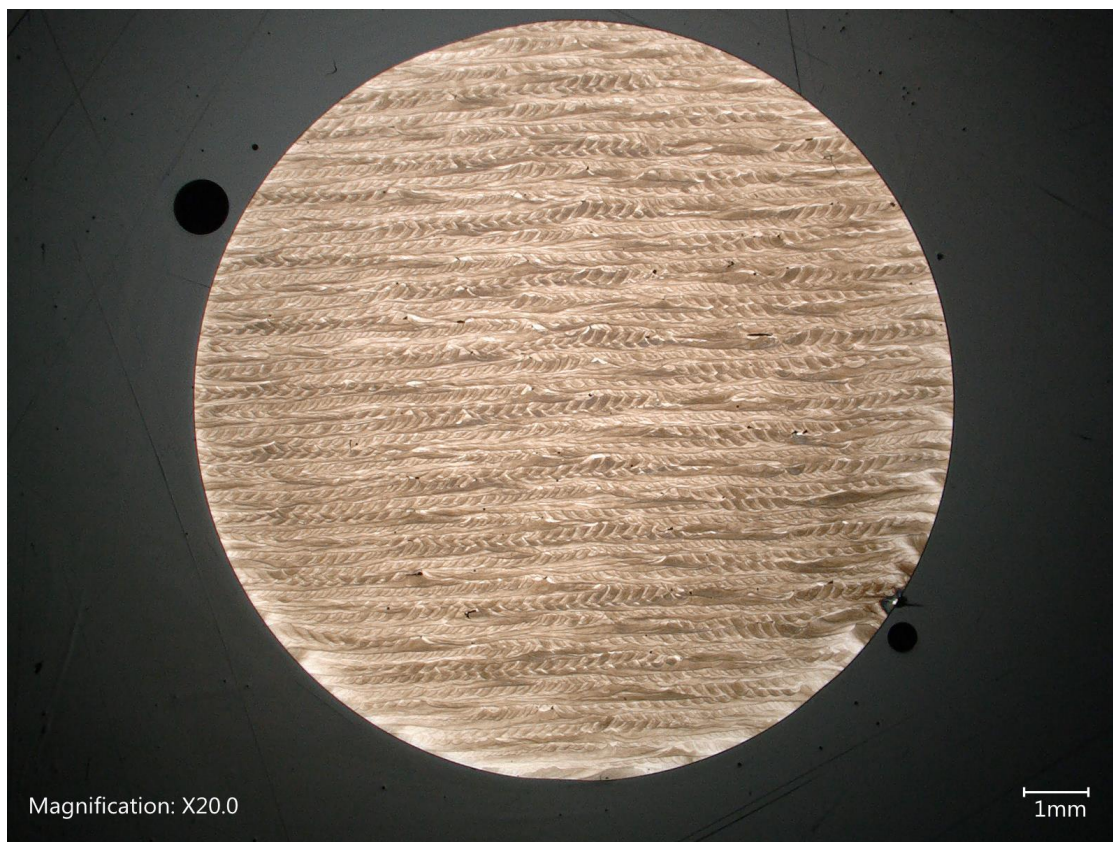
Figure 12. Melt pool structure observed at a 45^\circ cross-section of an as built AM U-6Nb specimen imaged via optical microscopy
