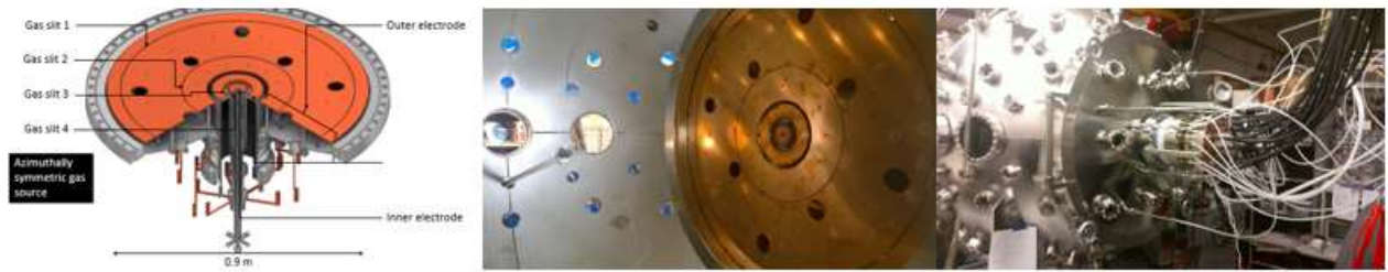
Fig. 13: (left) Design of the Mochi.LabJet.Gun with azimuthally symmetric gas slits and three electrodes (inner, middle, and outer electrodes). (middle, right) Photographs of the gun mounted on the spherical vacuum chamber. The gas slits are designed to allow free rotation of the plasma jet. The three electrodes are designed to mimic rotation shear on accretion disks to form a core and skin plasma jets.
