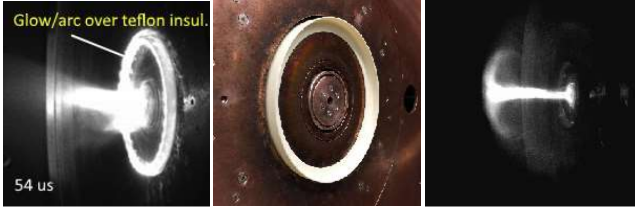
Fig. 22: (left) glowing arc over the teflon insulator after the plasma jet detaches. The bank continues to power the discharge for another 50 \mu\text{s} but only the glow and a faint diffuse plume is visible; (middle) alumina insert designed to replace the teflon and prevent arcing; (right) image of the plasma jet after the alumina insert in position. The jet behaves similarly to the first campaign but following the detachment, a second, longer lasting jet forms (Fig. 8).
