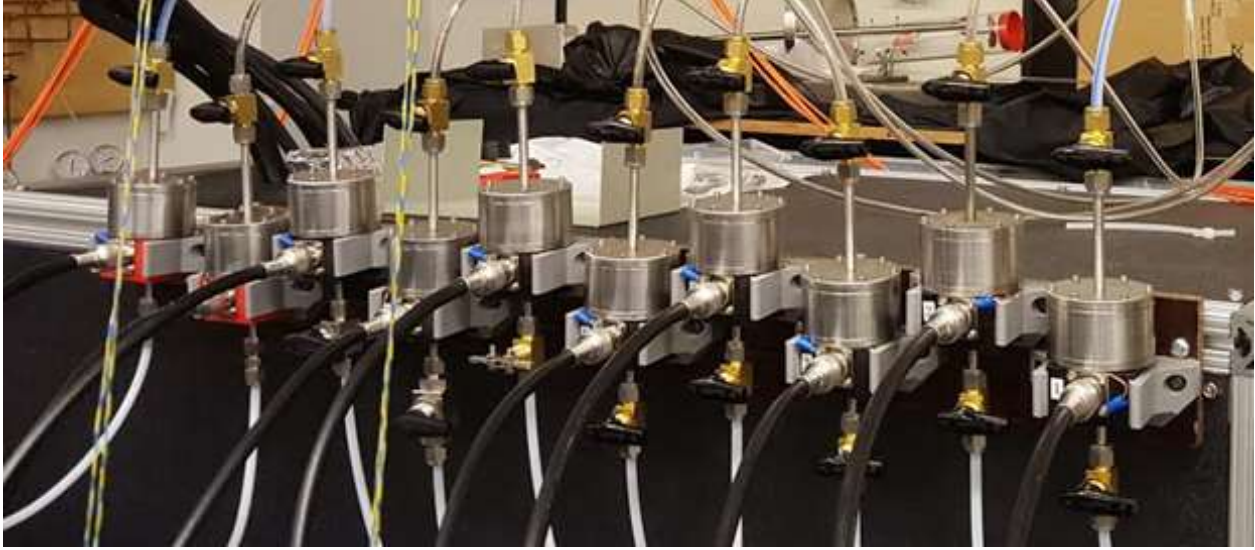
Fig. 17: Custom fast gas valves manufactured in house that can deliver 10^{21} particles each in 100\ \mu\text{s} time scales. These valves are necessary for delivering sufficiently dense gas close to the electrodes for breakdown without having to pre-fill the vacuum chamber. This allows formation of dense plasma jets inside a vacuum and not inside a background gas.
