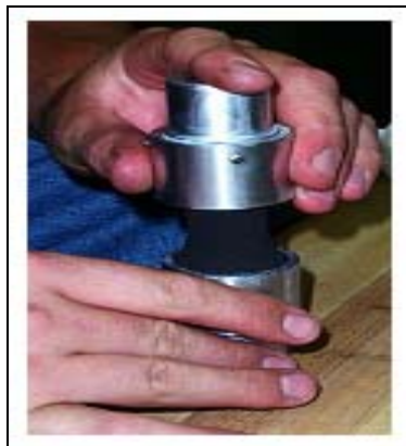
Figure 2.18 Assembled Specimen for Tensile Test
