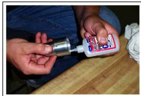
Figure 2.16 Placing Superglue in End cap
