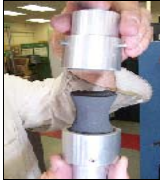
Figure 2.19 Tensile Failure of Sample 16of36
