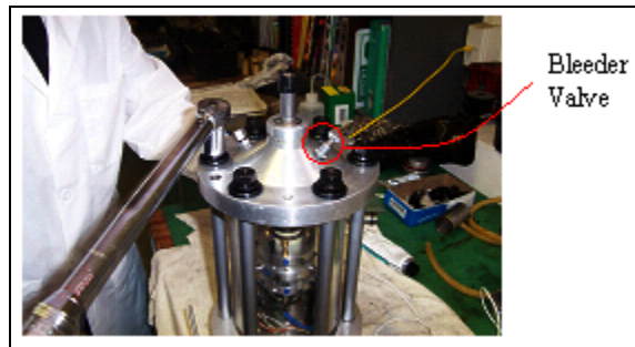
Figure 2.11 Assembled Triaxial Compression Cell
