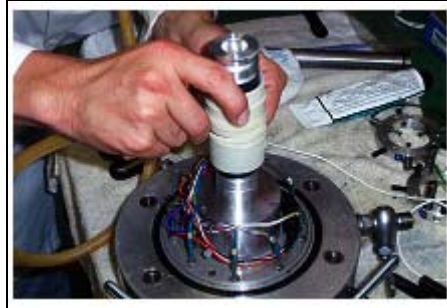
Figure 2.4 Placement of Rubber Membrane over Sample
