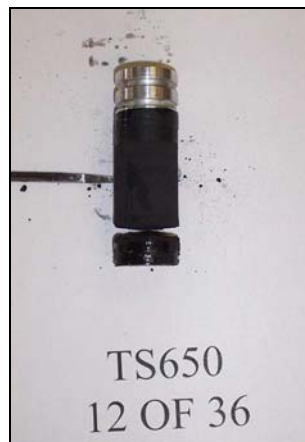
Figure 2.14 Fracture Angle for Sample 12of36
