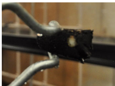
Magnesium Hydroxide 23.7 wt% After 5 second burn
