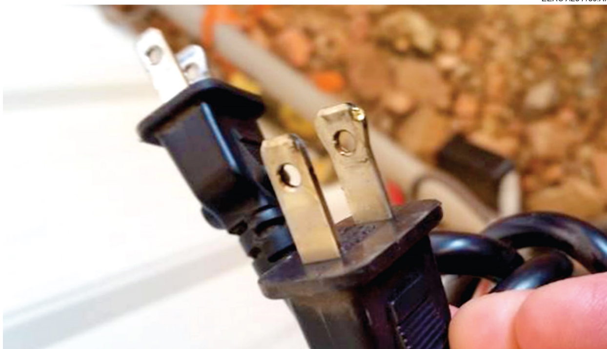
Figure 12. Melted metal observed on equipment plugs after the surge at the source shed.
