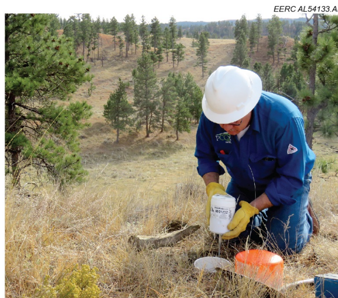
Figure 6. Semipermanent installation of the node array: nodes were placed within dug-in PVC sleeves and protected by a PVC cap.
