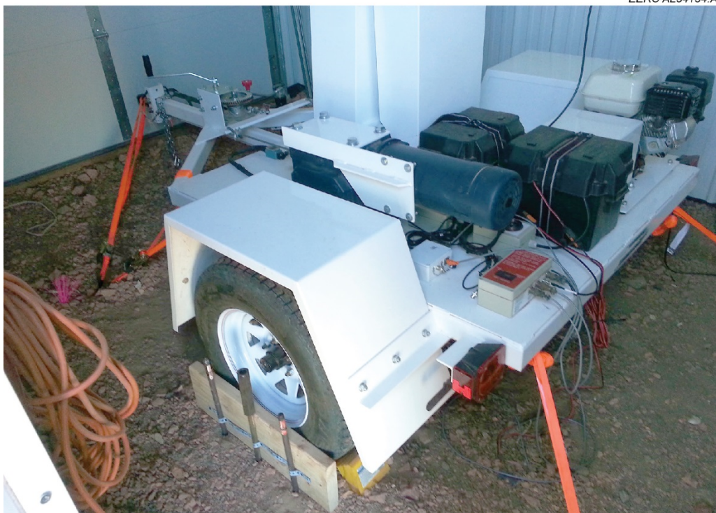
Figure 7. The seismic source was secured in a semipermanent manner to minimize movement and ensure a consistent source signature.
