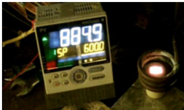
Figure 4-2. Heating application laboratory test with F/M steel using induction power supply, 3-turn helical coil, and a temperature controller.
