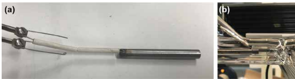
Figure 8-47. (a) The actual cladding tube directly attached with the thermos couple by using a spot welder. (b) The sample loaded at front of the nozzle in the reaction chamber.
