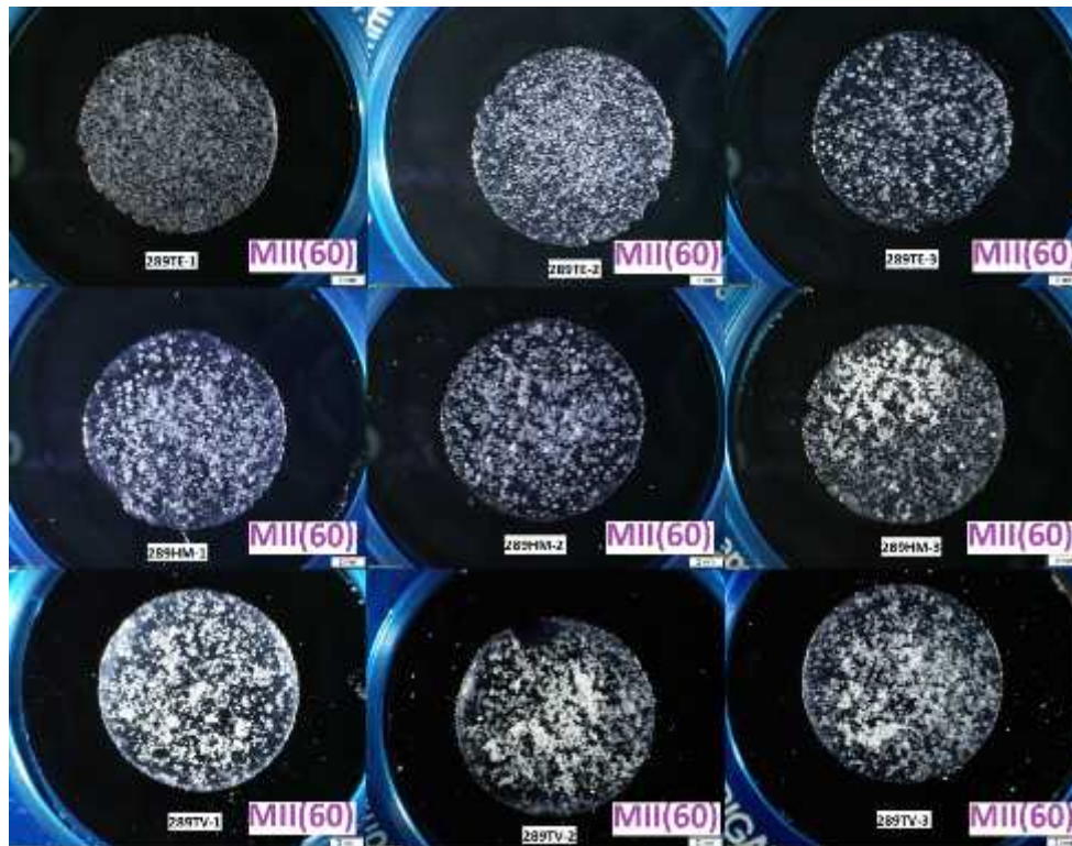
Figure AI-10. Thermonatrite specimen preparations.
