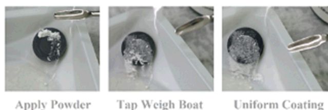
Figure 12. Method I - Powder deposition using a microspatula is illustrated in this composite figure advancing from left to right.
