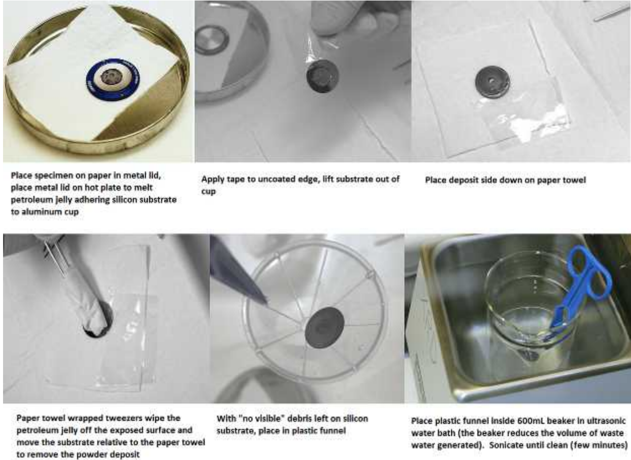
Figure AIV-3. This composite image illustrates the sequence of operations used to safely recover re-useable specimen mount components.
