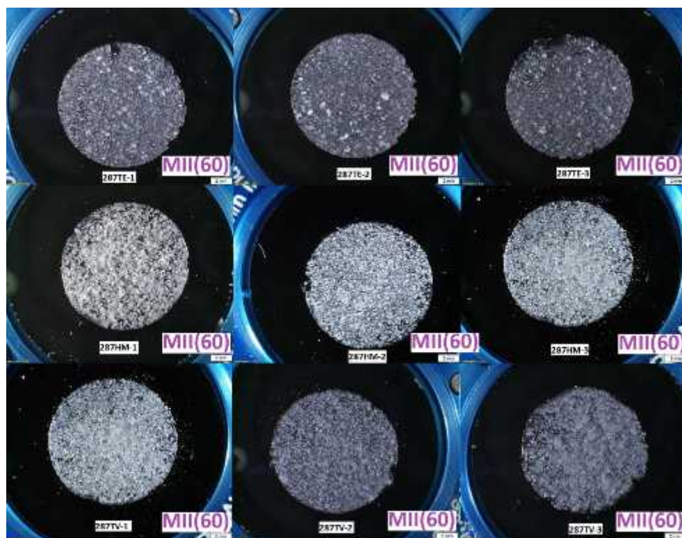
Figure AI-6. Burkeite specimen preparations.
