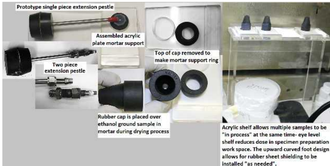
Figure AIV-2. Specialized tools developed for XRD specimen preparation are shown in this composite image. (Upper left to lower left): Prototype and follow-on design extension pestles; (Upper center to lower center): Mortar support plate components; (Right): Acrylic shelf with upper drying rack, lower area for solid waste and specimen storage under black rubber sheet shielding.
