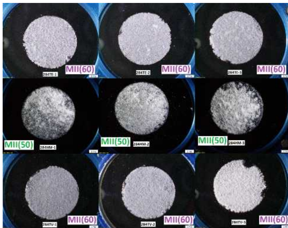
Figure AI-2. Natroxalate specimen preparations.
