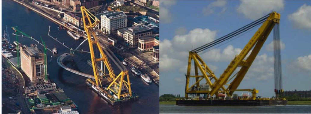
Figure 11. Asian Hercules II shearleg crane, with (left) and without (right) luffing jib.
