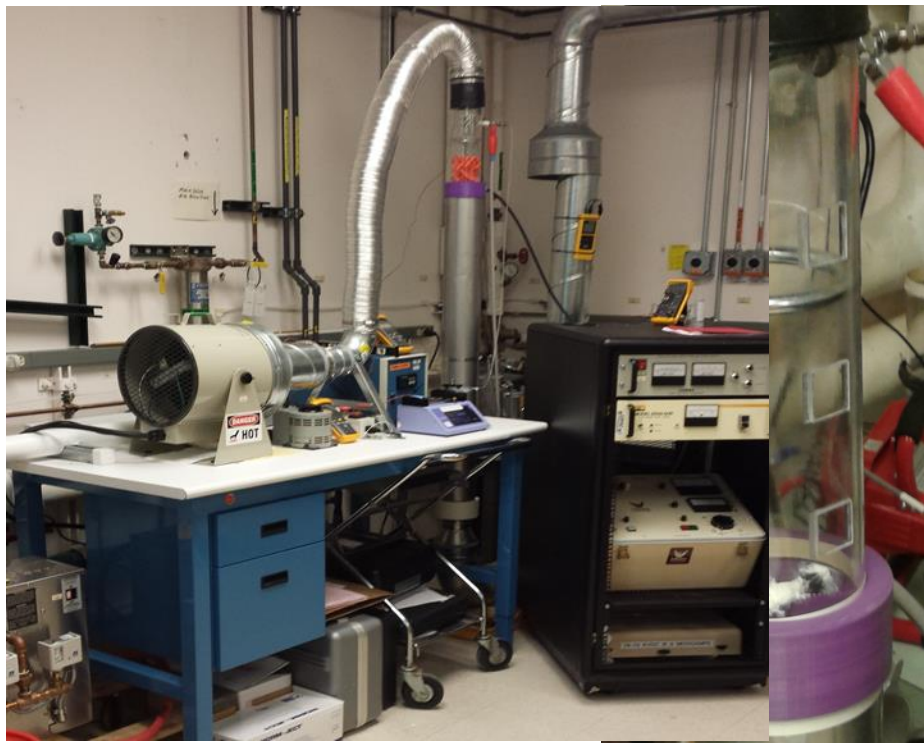
Figure 6 View of fully instrumented, integrated test system with enlargement of nebulizer and ESP to right (orange mixers removed)
