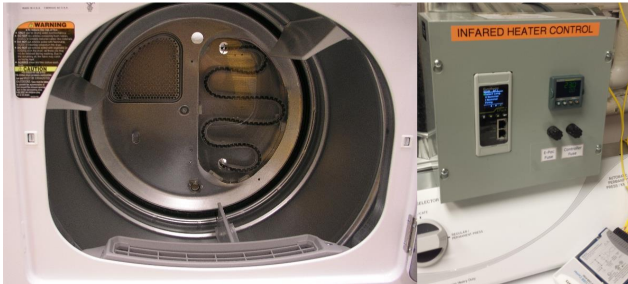
Figure 9 Installed IR heater in dryer drum left, IR heater controller right.
