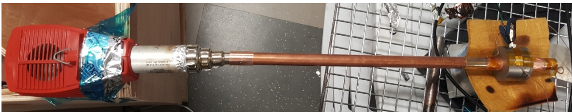
Figure 3.13: Experimental setup using heat gun with two settings. Extension is changed to obtain temperature variation.
