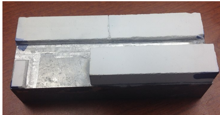
Figure 2.39: Preparation of machinable alumina for the CNC fabrication.
