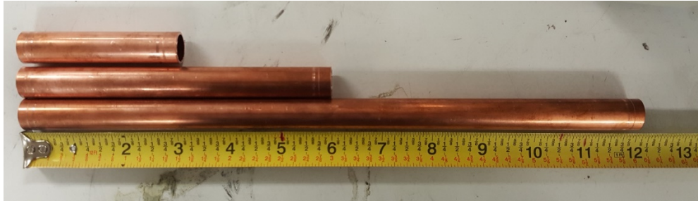
Figure 3.12: copper tube extensions to test temperature variation on the test tube. Three settings were tested: 3 in, 6 in, and 12 in.
