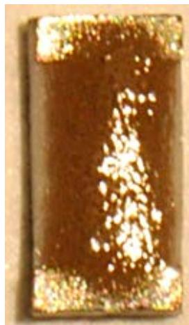
The figures are three views of single field-structured chemiresistor. This extremely small version of an FSCR was the latest generation of its kind developed during this CRADA project.
