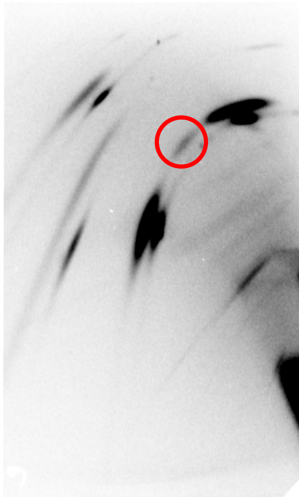
Figure 1. Diffraction image for shocked tantalum, showing twinning feature (circled).
