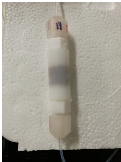
Figure 6. 1-inch mini-column with (1 gram of dolomite + fittings).
