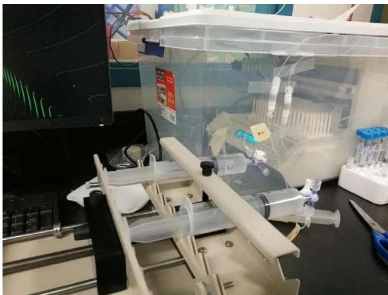
Figure 8. Image of the experimental setup for Cs experiments with two syringes (one for stressed and one for viable bacteria) connected to syringe pump and injected into columns with effluent collection in the fraction collector in a makeshift humidity chamber.
