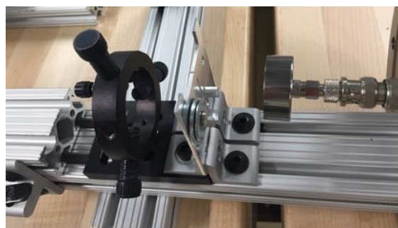
Fig. 9: Schematic (left) and experiment setup (right) of energy loss measurements of fission fragments from Cf-252 through carbon conversion foils from the TOF setup and through SiN windows used on the ionization chamber.
