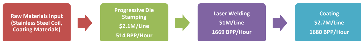
Figure 2-2: Bipolar plate process flow. Production rates refer to welded bipolar plate assemblies with flow fields on the anode and cathode sides and coolant channels between.
