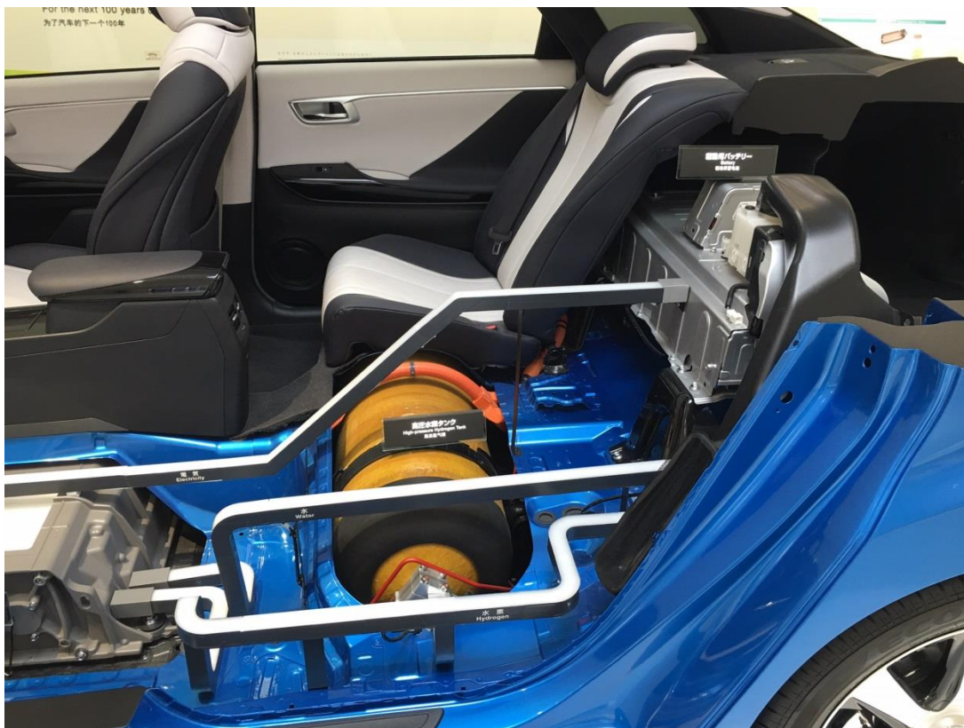
Figure 9-5: One of two 700 bar Type IV H 2 pressure vessels on the Toyota Mirai (source: Patrick Fullenkamp).
