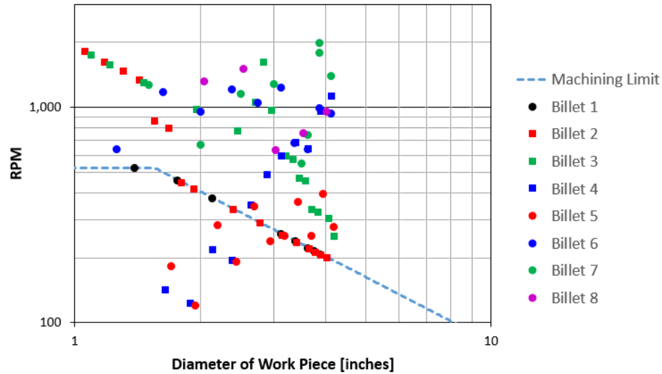
Figure 4.1. Experimental Machining Points in Reference to Safety Limit for PBX 9501
