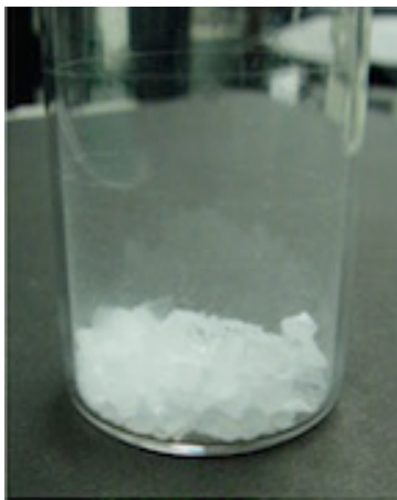
Figure 7: A silica gel after drying by direct evaporation. Gel breaks into small pieces.
